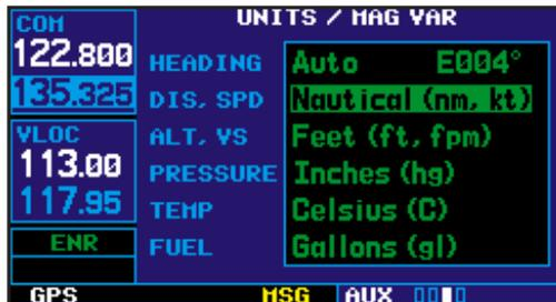
The *setup 1* page provides access (via “menu options”) to airspace alarms, CDI scale adjustment, an arrival alarm, units of measure settings, position formats, map datums and settings for local or UTC time display. When a menu option is selected, the corresponding page will appear providing access to the various unit settings.
