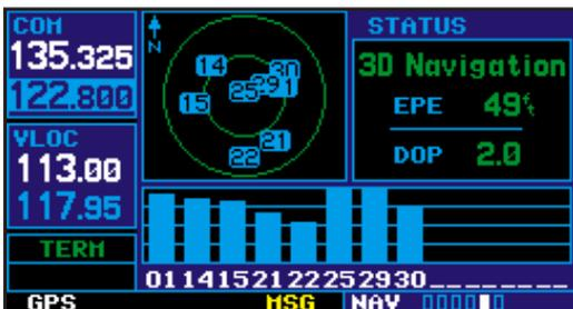
To switch the active and standby frequencies, press the **C** key. Switching the active and standby frequencies will not remove the cursor from the COM window.
