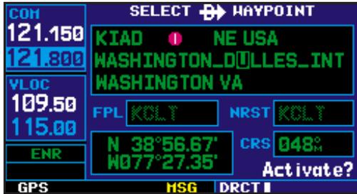
To select the direct-to destination by facility name (shown above) or city location (shown below), highlight the second or third line on the direct-to waypoint page. Use the small (PUSH CRN) and large (PUSH CRN) right knobs to enter the facility name or city. The identifier(s) for any matching entries will appear on the top line of the page.
