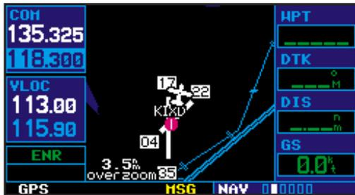
Once the standby frequency is selected, use the (⌚) (flip-flop) key to make the frequency active for transmit and receive operations.
