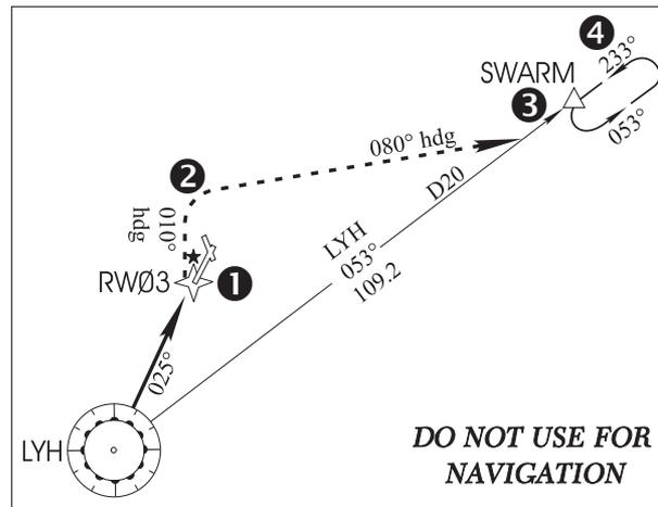
1. Press the **OBS** key. The missed approach holding point (MAHP; in this case "SWARM" intersection) is automatically offered as the destination waypoint.
