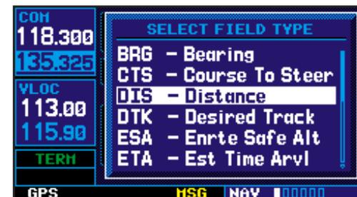
The large right knob (⊕) is used to select the data field you wish to change. Then use the small right knob (⊖) to display a list of data options and select the desired data item.
