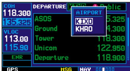
The navigation/communications (NAVCOM) page provides a complete list of airport frequencies at your departure, en route and arrival airports. To place a frequency from this list on standby, highlight the desired frequency and press **ENT**.
