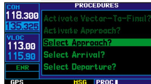
Press the **PROC** key to display the procedures page. Rotate the large right knob (CRSB) to select the desired option.
