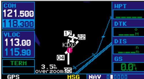
Press and hold the
