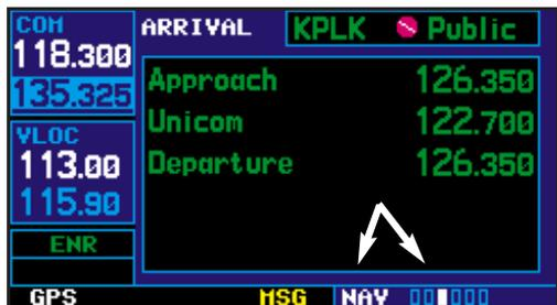
The bottom right corner of the screen indicates which page group is currently being displayed (e.g., NAV or NRST), the number of screens available within that group (indicated by square icons) and the placement of the current screen within that group (indicated by a highlighted square icon). To select a different page within the group, rotate the small right knob (PUSH CLR).
