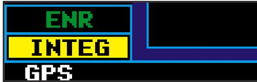
An 'INTEG' annunciation at the bottom left corner of the screen indicates that satellite coverage is insufficient to pass built-in receiver autonomous integrity monitoring (RAIM) tests. When this occurs, the GPS receiver will continue to provide navigation information, but should not be used for primary navigation guidance. Use the GNS 430's VLOC receiver or another suitable navigation source.
