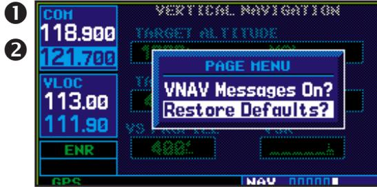
GPS accuracy may be degraded by the U.S. Department of Defense-imposed Selective Availability (SA) program. With “SA” on, GPS altitude may be in error by several hundred meters. Errors of this magnitude may result in fluctuations in the VSR readout on the default NAV page.
