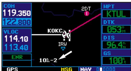
The **CLR** key allows you to quickly declutter the map display, providing four levels of map detail. Note the “-1” and “-2” (“-3” is also provided) suffix designations above, indicating each successive declutter level.
