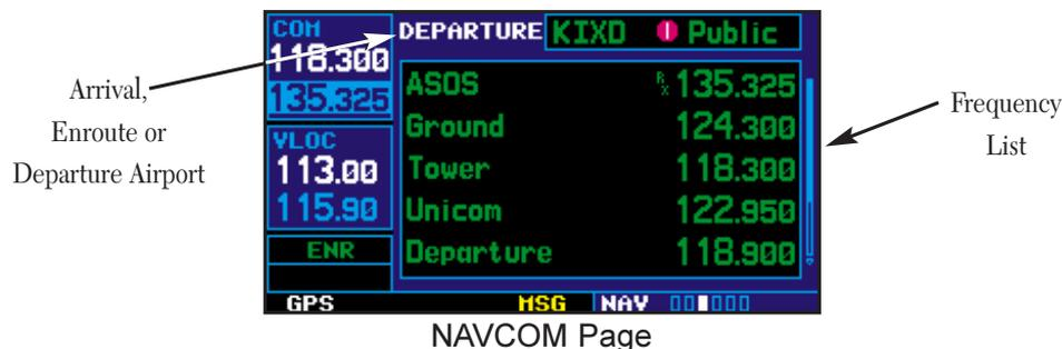
A frequency listed on the NAVCOM page can be quickly transferred to the standby field of the COM or VLOC windows. This time saving process prevents having to “re-key” a frequency already displayed elsewhere on the screen.
