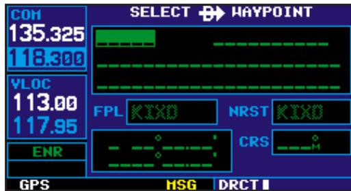
Data is entered using the large and small knobs. Experiment with them to become efficient at entering data. This will greatly reduce the amount of time spent operating the GNS 430 in flight.
