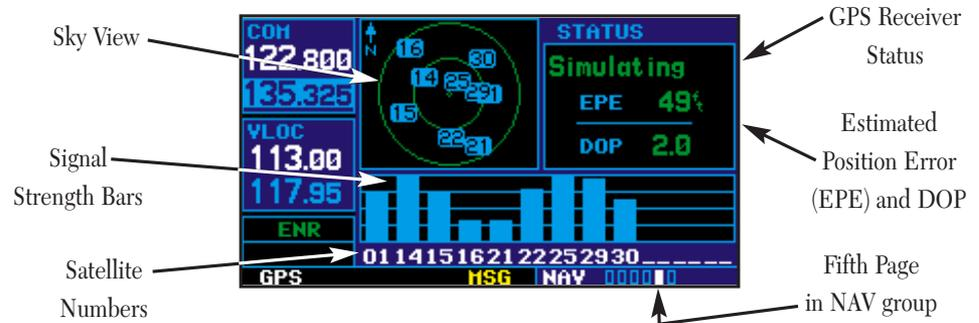
As the GPS receiver locks onto satellites, a signal strength bar will appear for each satellite in view, with the appropriate satellite number (01-32) underneath each bar. The progress of satellite acquisition is shown in three stages:
