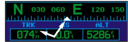
The graphic “track” indicator and the TRK indication directly below it provide the same information. Use the graphic “track” indicator for quick at-a-glance ground track information.
