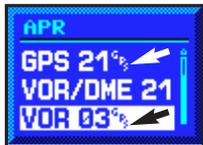
Not all approaches in the database are approved for GPS use. As you select an approach, a “GPS” designation to the right of the procedure name indicates the procedure can be flown using the GPS receiver. Some procedures will not have this designation, meaning the GPS receiver may be used for supplemental navigation guidance only. ILS approaches, for example, must be flown by tuning the VLOC receiver to the proper frequency and coupling the VLOC receiver to the external CDI (or HSI).
