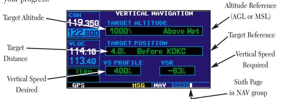
**NOTE** To use the vertical navigation features, your ground speed must be greater than 35 knots and you must be navigating to a direct-to destination or using a flight plan.
