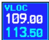
The GNS 430 includes digitally-tuned VOR/localizer and glideslope receivers with the desired frequency selected on a *VLOC window*, along the left-hand side of the display. Frequency selection is performed by pressing the small left knob (PUSH C/V) and rotating the small (PUSH C/V) and large (PUSH C/V) left knobs to select the desired frequency.
