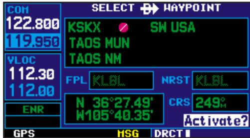
Confirm the selected direct-to destination by highlighting “Activate?” and pressing **ENT**.
