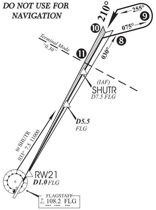
8. Turn right to a heading of 075° to initiate the procedure turn. The GNS 430 will not guide you through the turn. (The procedure turn is displayed on the map page and indicated as the active leg on the default NAV and active flight plan pages.) The external CDI needle will start moving to the left.
