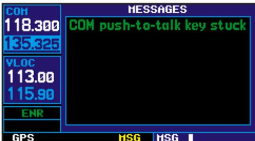
A “COM push-to-talk key stuck” message appears to warn you of a stuck microphone. Transmitting is disabled after 35 seconds of continuous broadcasting.
