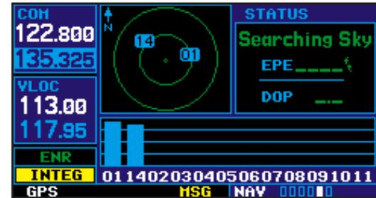
The *satellite status page* shows the ID numbers for the satellites and the relative signal strength of each satellite received (as a “bar graph” reading).
