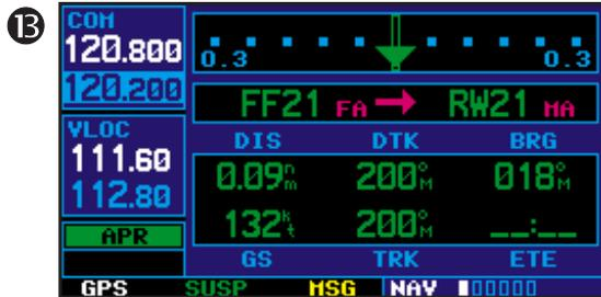
9. At 2.0 nautical miles from the FAF (FF21; a Jeppesen-provided waypoint), the GNS 430 will switch from terminal mode to approach mode. CDI scaling will be tightened from 1.0 to 0.3 nautical mile, full scale deflection.
