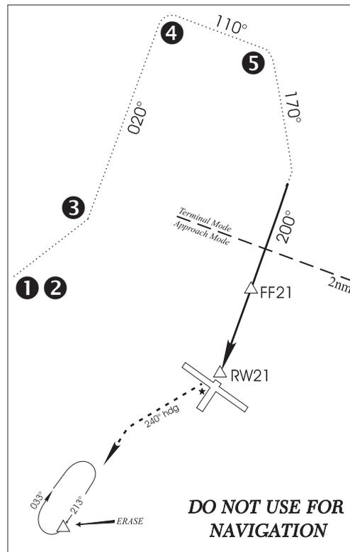
1. Within 30 nautical miles of KFOE, the GNS 430 will switch from enroute mode to terminal mode and the CDI scale will transition from 5.0 to 1.0 nautical miles, full scale deflection.
