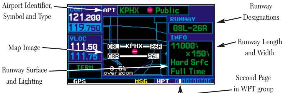
The *airport runway page* displays runway designations, length, surface type and lighting for the selected airport. A map image of the runway layout and surrounding area is also displayed on the *airport runway page*. The map image scale appears in the lower left corner and is adjustable using the **▽ RNG △** key. For airports with multiple runways, information for each runway is available.
