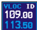
VLOC ident is enabled by pressing the V knob. When VLOC ident is enabled, an “ID” indication appears in the upper right corner of the VLOC window — to the immediate right of “VLOC”.
