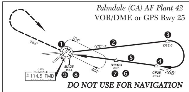
1. As you reach the initial approach fix (PMD), a waypoint alert ("NEXT DTK 070°") will appear in the lower right corner of the screen. As the distance to the IAF approaches zero, the alert is replaced by a turn advisory ("TURN TO 070°"). Dial the outbound course into the CDI (or HSI) using the OBS knob and initiate a standard rate turn to this course heading.
