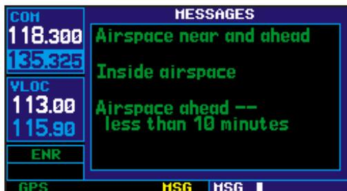
When an airspace alert occurs, the message (MSG) annunciator will flash. Press **MSG** to view the alert message.
