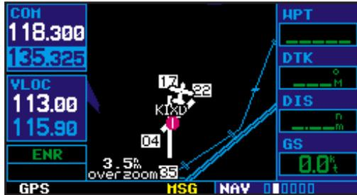
Tuning cursor in the COM window. Use the small (⌚) and large (⌚) left knobs to dial in the desired standby frequency.
