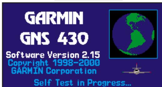
The welcome page appears when the GNS 430 is turned on. During the time this screen is displayed, the GNS 430 performs a self-test to ensure proper operation.
