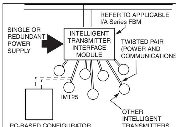
Figure 5. Functional Block Diagram FoxCom Digital Output Only
