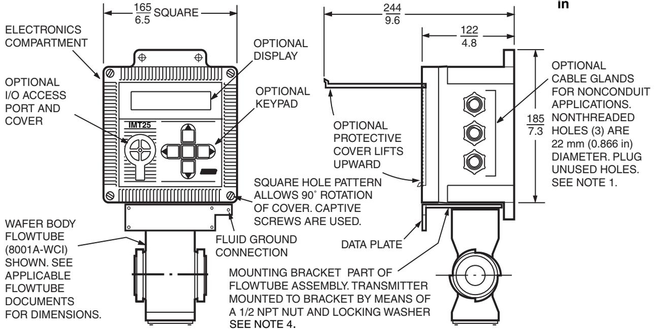
**FLOWTUBE MOUNTED TRANSMITTER - OPTIONAL DUAL COMPARTMENT**
