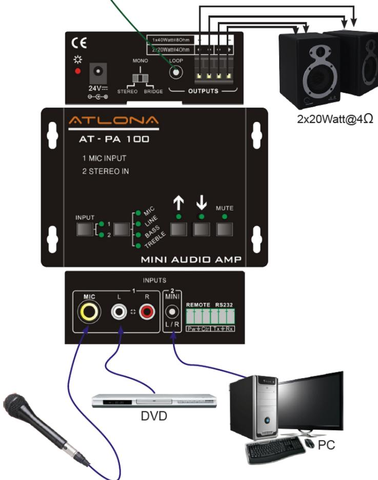
\* The "loop" out port allows a source to pass-through to another device.
