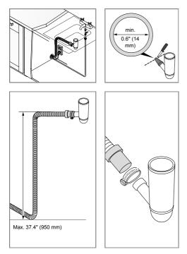
The drain hose can also be connected to a connection nipple on the sink unit's water trap. The connection nipple must have an internal diameter of at least 0.6" (14 mm).
