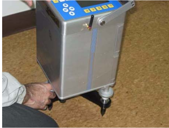
Figure 3-7 - Leveling the Tripod using the Front Footscrew
