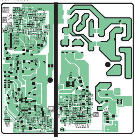
KX-FLM663CNS/KX-FLM663CNW LOW VOLTAGE BOTTOM VIEW
