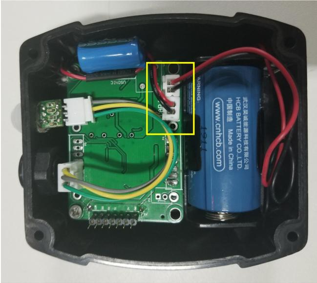
Figure 5.1 Connect battery and capacitor
