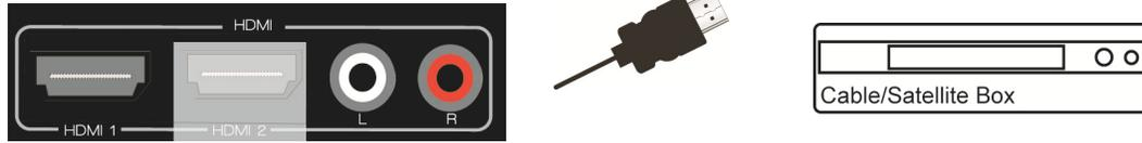
Cable and Satellite Boxes that have a HDMI digital interface should be connected using HDMI for optimal results. To maintain image quality, use a VIZIO certified HDMI cable. This cable is available in 6, 15, and 30 foot lengths. See [www.VIZIO.com](http://www.VIZIO.com) or call **877-MYVIZIO** (877-698-4946) for details.
