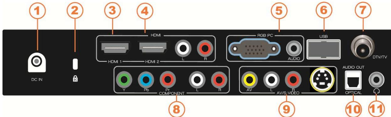
1. **DC IN**—Connect the included DC power supply here. Connect the other end to a wall outlet.
