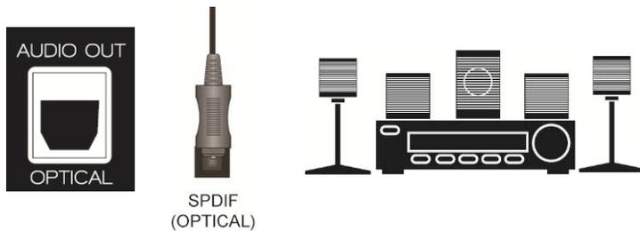
If your sound system has a SPDIF (optical) digital audio input you can connect it from your sound system to the **OPTICAL** digital audio out on the back of your HDTV. This is active when receiving audio with the programs being viewed no matter what input is being used.
