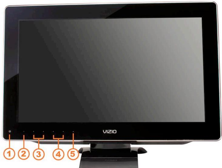
**5. INPUT (SELECT)**—Press to cycle through the various devices connected to your TV (called Inputs). The inputs cycle in the following sequence: TV, AV (Composite), COMP (Component), HDMI-1, HDMI-2, and RGB (VGA). Once you have stepped through the entire sequence, you will return to the beginning. If a sub-menu is active, pressing this button will return to the previous menu level. Additionally, when the menu is active, this button confirms the menu function to be adjusted.
