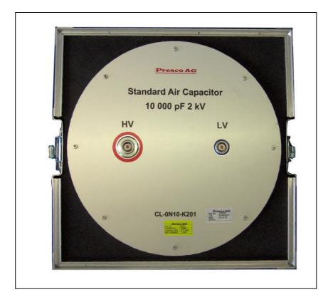
Connect the HV connector by a LEMO connector and 2 kV cable to HV source as it described above.
