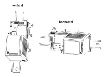
Use the optional 1794-CE1 (0.3m, 1ft) or 1794-CE3 (0.9m, 3ft) extender cable to add an extended-local rail of I/O to the controller. You can have as many as eight I/O modules on the local rail and eight modules on the extended-local rail.
