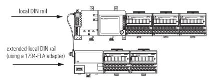
When you create a project for a FlexLogix controller, the Controller Organizer for that project automatically displays both the local DIN rail and the extended DIN rail. If you do not use the extended-local DIN rail, inhibit that rail.
