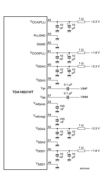
Fig.5 PLL and ADC connections.
