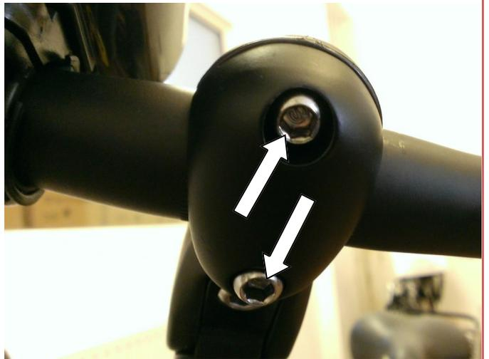
To adjust the **rotation** of the handlebars (to ensure that the angle of the brakes/display etc. is correct), loosen the front-most bolt on the underside of the handlebars as shown above right. Rotate the handlebars into the desired position and then re-tighten the bolt. Check the adjacent bolt is sufficiently tight and tighten if required.
