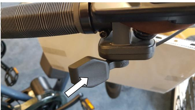
Try to ensure that the bike is in a low gear when starting off, this will reduce the strain on the motor and extend its life. Regularly starting off in a high gear may damage your motor and would not be covered by the warranty.
