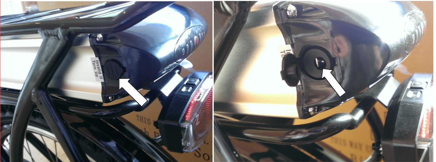
To charge the battery, simply lift the weatherproof cover and connect the charger to the socket and then plug the other end into a regular mains socket. On the charger is a small light which is red while charging. When charging is complete, this light will turn green.
