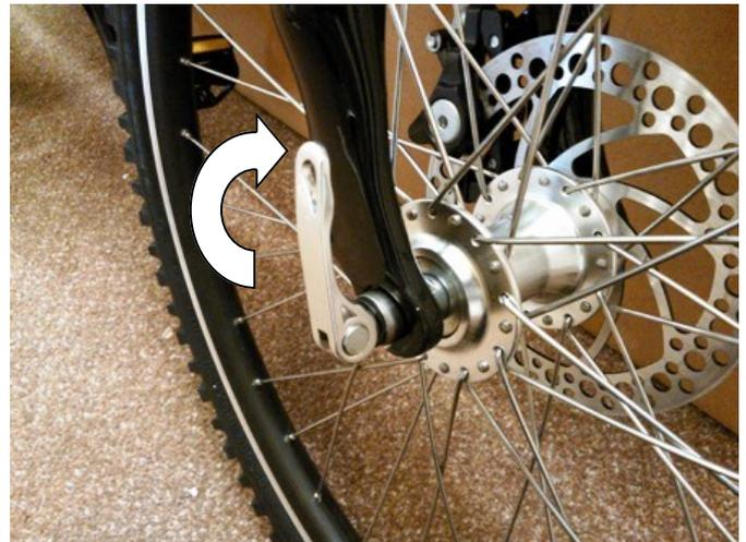
Now that the front wheel has been fitted, you can flip the bike right side up and use the kick-stand to keep the bike in the upright position.
