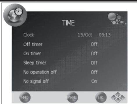
This adjustment allows you to set or to display the following functions: Clock, Off / On Timer and Sleep Timer.
