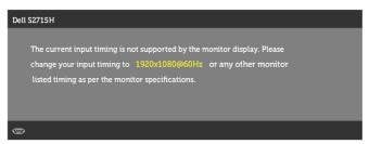
This means that the monitor cannot synchronize with the signal that it is receiving from the computer. See Monitor Specifications for the Horizontal and Vertical frequency ranges addressable by this monitor. Recommended mode is 1920 x 1080.
