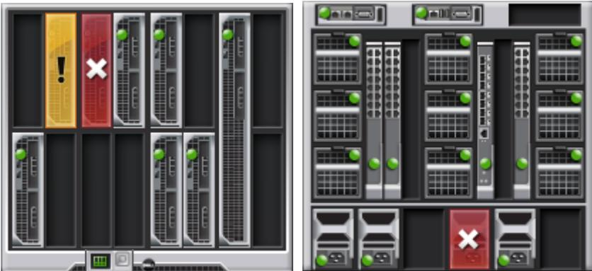
The **Chassis Health** page provides an overall health status for the chassis, active and standby CMCs, server modules, IO Modules (IOMs), fans, iKVM, power supplies (PSUs), and LCD assembly. More detailed information for each component is displayed by clicking on that component. For instructions on viewing chassis and components summaries, see "Viewing Chassis Summaries" on page 392.
