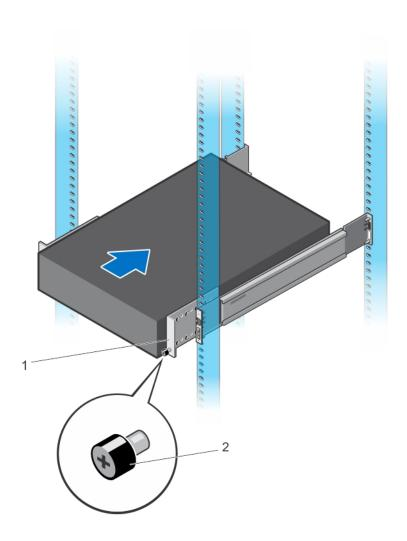
Figure 18. S5296F-ON installation
