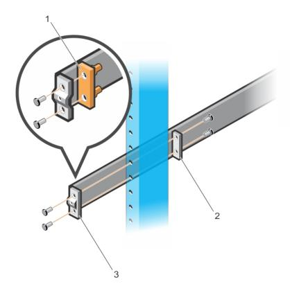
Figure 13. Two-post flush-mount installation
