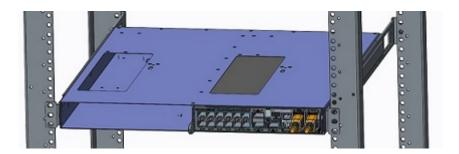
Figure 7. Install one-half U switch
