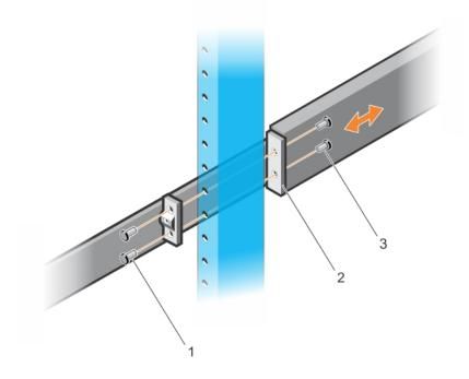
Figure 14. Two-post center-mount installation
