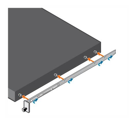
Figure 16. Switch rail attachment
