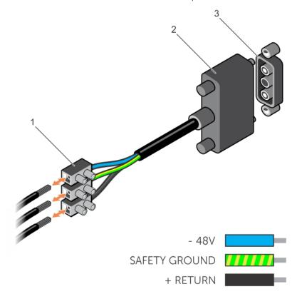
Figure 21. DC power connector and wiring block
