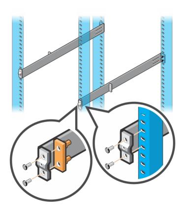
Figure 15. Four-post threaded installation
