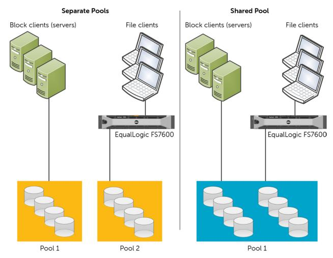
Figure 2 Logical diagram for separate or shared pool
