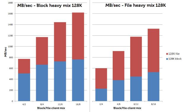
Figure 5 Throughput (MB/sec) with 128K I/O request in shared pool
