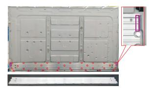
Use a screwdriver to remove18pcs screws for unlocking the two VESA brackets with back bracket.(Torque: 5±0.5kgf)
