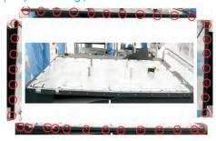
Use a screwdriver to remove 15pcs screws for unlocking H-beam with the assembled unit, and then S13 remove the H-Beam.
