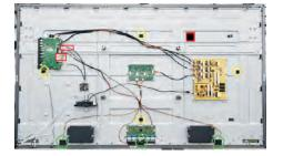
Disconnect all the cables as the picture below shown. S7 Use a screwdriver to remove 2pcs screws for unlocking AC power outlet.(Torque: 4.5±0.5kgf)
