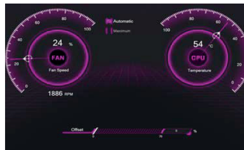
Figure 9 - Fan Speed Control
