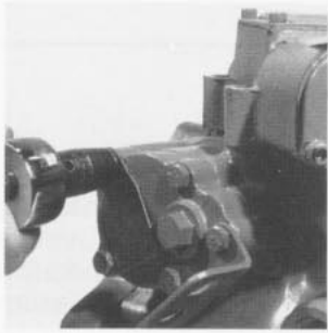
Fig. 15 - Remove Servo Cover (Opposite Neutral Adjustment)
