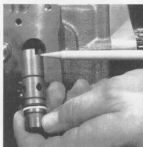
Fig. 83 - Slot in Control Sleeve
