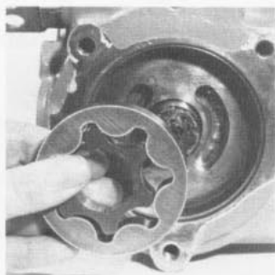
Fig. 50 - Install Gerotor Assembly
