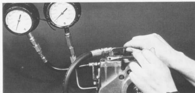
Fig. 21 - Adjusting Swashplate Neutral
