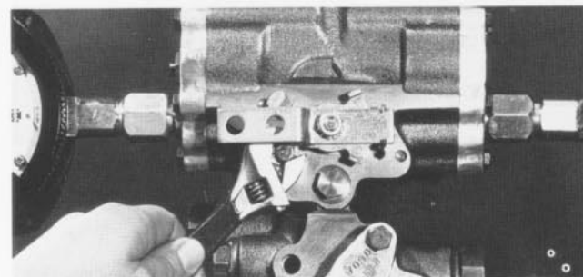
Fig. 23 - Loosen Neutral Bracket Retaining Screw
