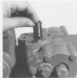
Fig. 89 - Remove Control Sleeve
