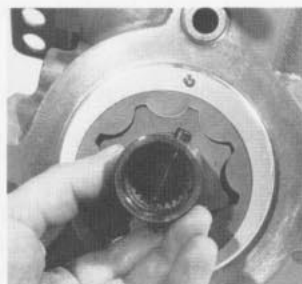
Fig. 66 - Install Drive Coupling (Earlier Units)
