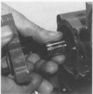
Fig. 17 - Install Spacer and Replace Cover
