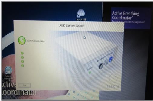
Figure 26 : ABC System Check should all be green (connected).
