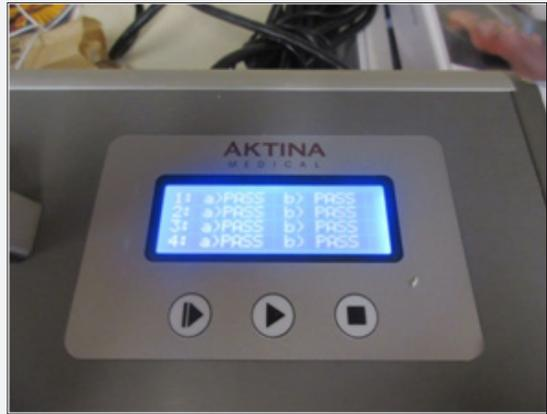
**Figure 15 :** The QA device will run tests and a prompt will come up and tell you if the test has passed or failed.
