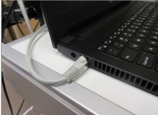
**Figure 8 :** Laptop Connection to ABC cart using the network cable.
