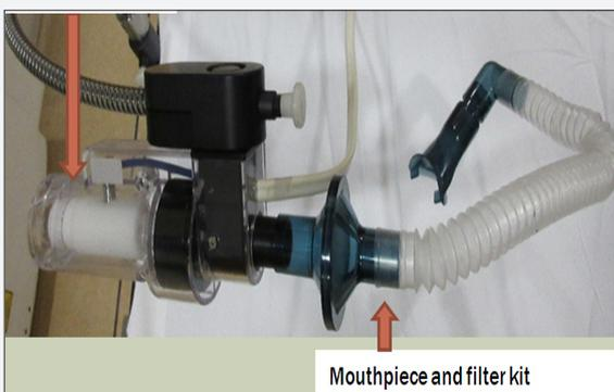
Figure 6 : Measures the quantity of air a patient breathes through the ABC system.
