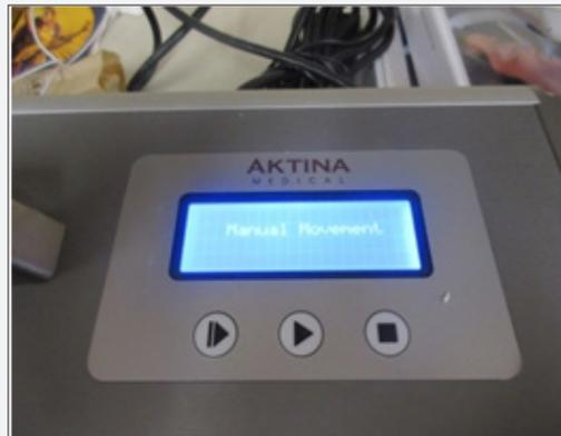
**Figure 16 :** Once the “automatic test” passes, scroll through the LCD menu to find the manual option.
