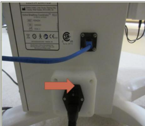
**Figure 39 :** Power switch for the ABC control cart is located on the side of the unit along with the network connector.
