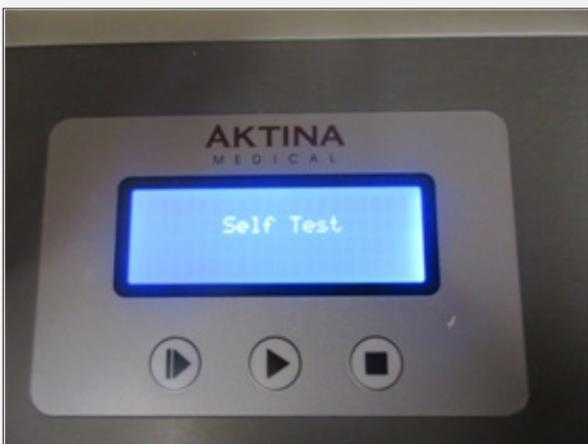
**Figure 14 :** Scroll down to “Self test “option on the LCD screen of the morning QA device.
