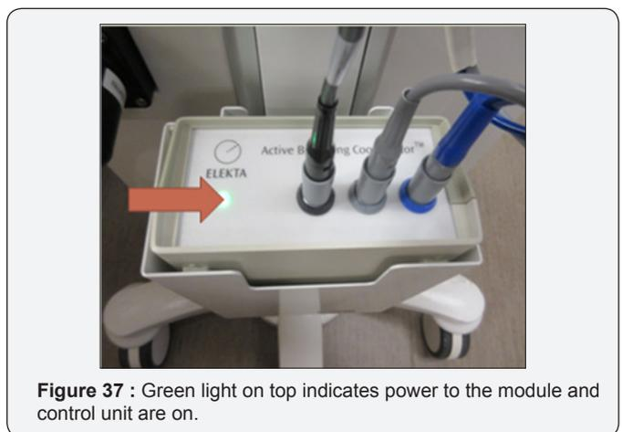
Figure 37 : Green light on top indicates power to the module and control unit are on.
