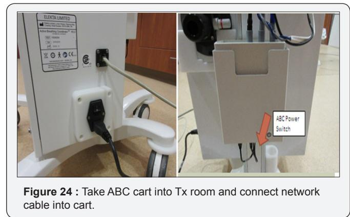
**Figure 24 :** Take ABC cart into Tx room and connect network cable into cart.
