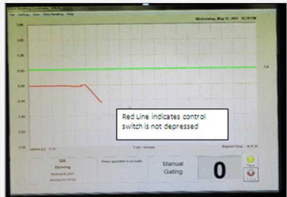
Figure 30 : Red Line Indicates control Switch is not depressed.
