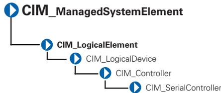
The CIM\_SerialController class explained in Table 3-26 contains controllers that transfer data one bit at a time to the devices they control, for example, a serial port controlling a modem.
