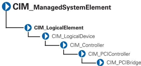
The CIM\_PCIBridge class shown in Table 3-29 describes the capabilities and management of a PCI controller providing bridge-to-bridge capability. An example is a PCI to Industry-Standard Architecture (ISA) bus bridge.
