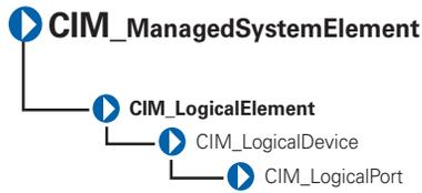
The **CIM\_LogicalPort** class listed in Table 3-14 represents the abstraction of a port or connection point of a device. For example, a USB port can be abstracted to represent a port. This feature is used when the abstracted port has independent management characteristics from the device that includes it.
