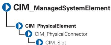
The CIM\_Slot class described in Table 2-11 represents connectors into which packages are inserted. For example, a physical package that is a hard drive can be inserted into a small computer system interface-single connector attachment (SCSI-SCA) slot. As another example, a card can be inserted into a 16-, 32-, or 64-bit expansion slot on a host board.
