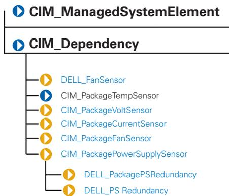
Each class derived from CIM\_Dependency has an element called an antecedent that represents the independent object in this association, and another element called a dependent that represents the object that is dependent on the antecedent. For example, consider two managed system elements: Chassis1 and PowerSupply3. Chassis1 is the antecedent element because a managed power supply would always be either contained in, or grouped with, a chassis.
