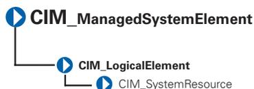
The CIM\_SystemResource class listed in Table 3-38 provides access to system resources from an operating system. SystemResources consist of interrupt requests (IRQs) and direct memory access (DMA) capabilities.
