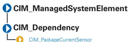
The CIM\_PackageCurrentSensor shown in Table 5-4 contains amperage sensors that are often installed in a package such as a chassis or a rack to assist in the monitoring of the package in general. This relationship is described by the CIM\_PackageCurrentSensor association.
