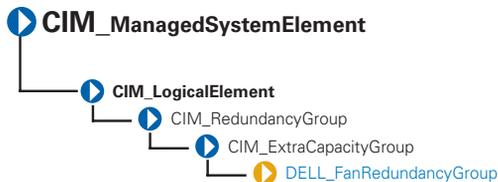
The DELL\_FanRedundancyGroup described in Table 3-45 defines what constitutes fan redundancy in a system.
