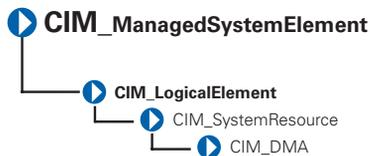
The CIM\_DMA class explained in Table 3-41 contains DMA information. A DMA channel allows certain types of data transfer between RAM and a device to bypass the microprocessor.
