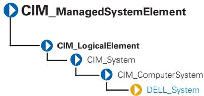
The DELL\_System class listed in Table 3-4 is the set of all Dell™ instrumented systems, including server and storage systems. For properties, see Table 3-2, "CIM\_System Properties."
