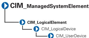
The CIM\_UserDevice class shown in Table 3-20 contains logical devices that allow a computer system's users to input, view, or hear data. Classes derived from CIM\_UserDevice include CIM\_Keyboard and CIM\_PointingDevice.
