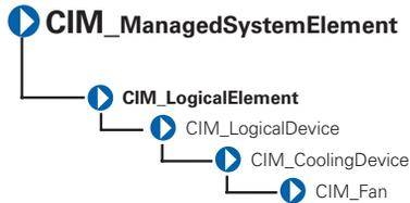
The CIM\_Fan class explained in Table 3-19 contains a set of devices that work to keep the ambient internal temperature of the system at a safe value by circulating air.
