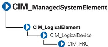
The CIM\_FRU class described in Table 3-6 contains manufacturing information related to the Field Replaceable Units (FRU) of a system such as a system planar or I/O riser card.
