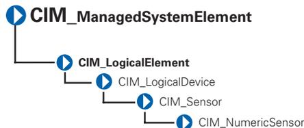
The CIM\_NumericSensor class described in Table 3-12 returns numeric settings and may also support threshold settings. Figure 3-2 shows the relationship among upper and lower critical and upper and lower noncritical threshold values. The normal range falls between upper and lower noncritical thresholds.
