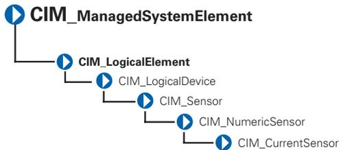
The CIM\_Sensor class explained in Table 3-10 contains hardware devices capable of measuring the characteristics of some physical property, for example, the temperature or voltage characteristics of a computer system.
