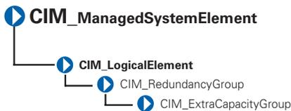
The CIM\_ExtraCapacityGroup class explained in Table 3-43 applies to systems that have more capability and components than are required for normal operation, for example, systems that have extra fans or power supplies.
