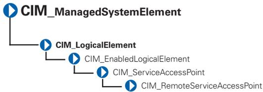
The CIM\_RemoteServiceAccessPointGroup class identified in Table 3-48 describes the accessing and addressing of information for a remote connection that is known to a "local" network element. This information is contained in the "local" network element since this is the context in which it is "remote". The relevance of the remote service access point and information on its use are described by subclassing or associating to the CIM\_RemoteServiceAccessPointGroup class.
