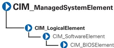
The CIM\_BIOSElement class listed in Table 3-35 describes the BIOS for the system. The BIOS controls the following:
