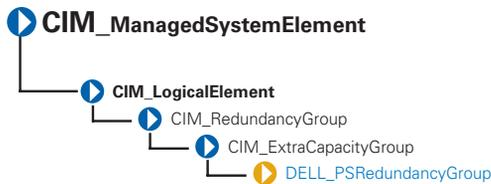
The DELL\_PSRedundancyGroup described in Table 3-44 is a Dell-specific extension of the CIM\_PowerSupply class. The DELL\_PSRedundancyGroup class defines what constitutes power supply redundancy in a system.
