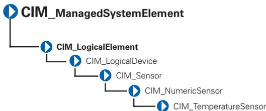
The CIM\_TemperatureSensor class listed in Table 3-13 contains sensors that sample ambient temperature and return a value in degrees Celsius.
