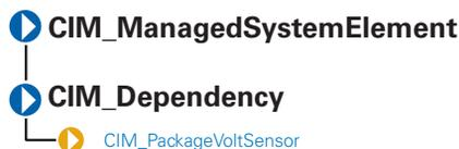
The CIM\_PackageVoltSensor identified in Table 5-3 contains voltage sensors that are often installed in a package such as a chassis or a rack to assist in the monitoring of the package in general. This relationship is described by the CIM\_PackageVoltSensor association.
