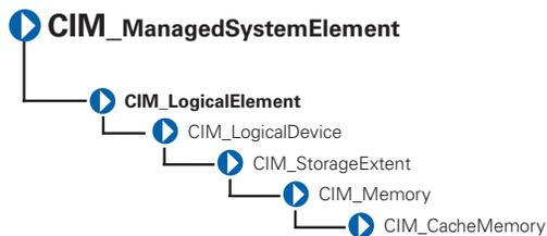
The CIM\_CacheMemory class explained in Table 3-33 describes the capabilities and management of cache memory. Cache memory allows a microprocessor to access data and instructions faster than normal system memory.
