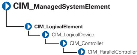
The CIM\_ParallelController class identified in Table 3-25 contains a set of objects that control parallel devices. Parallel controllers transfer 8 or 16 bits of data at a time to the devices they control, for example, a parallel port controlling a printer.
