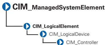
The CIM\_Controller class shown in Table 3-24 groups miscellaneous control-related devices. Examples of controllers are small computer system interface (SCSI) controllers, Universal Serial Bus (USB) controllers, and serial controllers.
