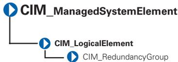
The CIM\_RedundancyGroup class explained in Table 3-42 is a set of components that provide more instances of a critical component than are required for the system's operation. The extra components are used in case of critical component failure. For example, multiple power supplies allow a working power supply to take over when another power supply has failed.
