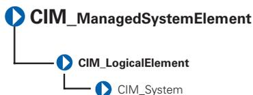
The CIM\_System class shown in Table 3-2 defines a collection of managed system elements that operates as a functional whole. An instance of the CIM\_System class contains a well-defined list of components that work together to perform a specific function.
