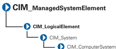
The CIM\_ComputerSystem class listed in Table 3-3 contains some or all of the following CIM\_ManagedSystemElements: file system, operating system, processor and memory (volatile and/or nonvolatile storage). For properties, see Table 3-2, "CIM\_System Properties."
