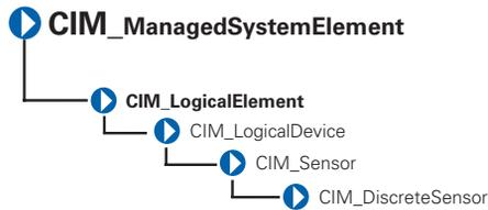
The CIM\_DiscreteSensor class described in Table 3-11 has a set of legal string values that it can report. The CIM\_DiscreteSensor will always have a "current reading" that corresponds to one of the enumerated values.
