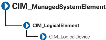
The CIM\_LogicalDevice class described in Table 3-5 models a hardware entity that may be realized in physical hardware. CIM\_LogicalDevice includes any characteristics of a logical device that manages its operation or configuration. An example of a logical device is a temperature sensor's reading of actual temperature.
