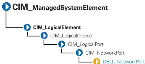
The DELL\_NetworkPort class listed in Table 3-9 represents the abstraction of a port or connection point of a device. For example, a USB port can be abstracted to represent a port. This feature is used when the abstracted port has independent management characteristics from the device that includes it.
