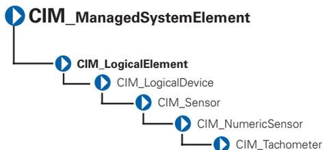
The CIM\_Tachometer class listed in Table 3-16 contains devices that measure revolutions per minute (RPM) of a fan and return the value in RPMs.
