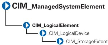
CIM\_StorageExtent identified in Table 3-31 contains devices that manage data storage, for example, hard drives or microprocessor memory.
