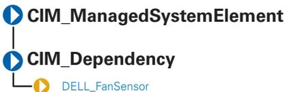
The DELL\_FanSensor class described in Table 5-1 defines a Dell-specific association between a fan and a sensor. The CIM\_PackageFanSensor class contains fans that assist in cooling the entire package as opposed to a fan that is dedicated to cooling only some of the components in the package.
