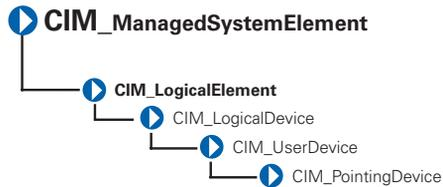
The CIM\_PointingDevice class described in Table 3-21 includes those devices used to point to regions of a display. Examples are a mouse or a trackball.
