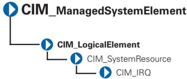
The `CIM_IRQ` class described in Table 3-39 contains `IRQ` information. An `IRQ` is a signal that data is about to be sent to or received by a peripheral device. The signal travels by an `IRQ` line to the microprocessor. Each peripheral connection must be assigned an `IRQ` number. For example, the first serial port in your computer (COM1) is assigned to `IRQ4` by default.
