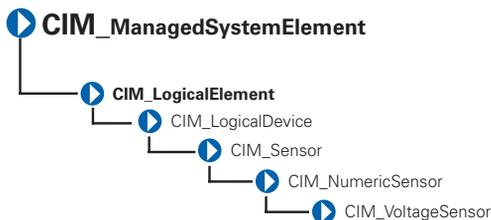
The CIM\_VoltageSensor class shown in Table 3-15 contains sensors that measure voltage and return a value in volts.
