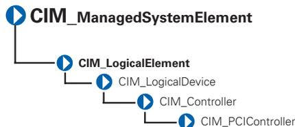
The CIM\_PCController class listed in Table 3-27 contains a set of devices that follow the Peripheral Component Interconnect (PCI) protocol defined by the Personal Computer Memory Card International Association (PCMCIA). The PCI protocol defines how data is transferred between devices. The CIM\_PCController class contains PCI adapters and bridges.
