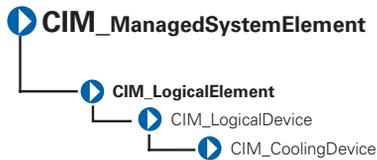
The CIM\_CoolingDevice class described in Table 3-18 contains a set of devices that work to keep the ambient internal temperature of the system at a safe value.
