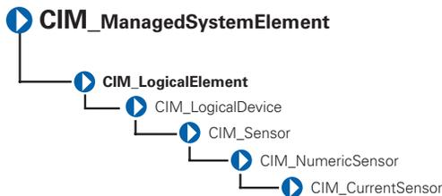
The CIM\_CurrentSensor class listed in Table 3-14 contains sensors that measure amperage and returns a value in amperes.
