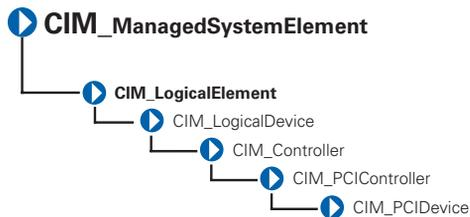
The CIM\_PCIDevice class shown in Table 3-28 describes the capabilities and management of a PCI device controller on an adapter card.
