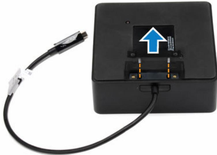
5. Pull out the USB Type-C cable from its connector inside the docking station.
