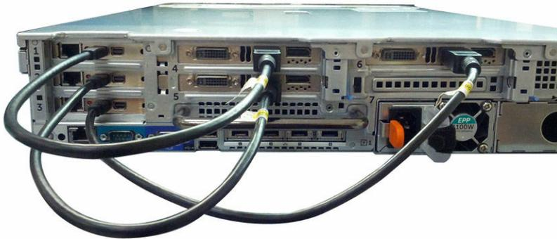
2. Connect the mini DisplayPort to DisplayPort cables from port 3 on the GPUs to port 2 on the host cards.
