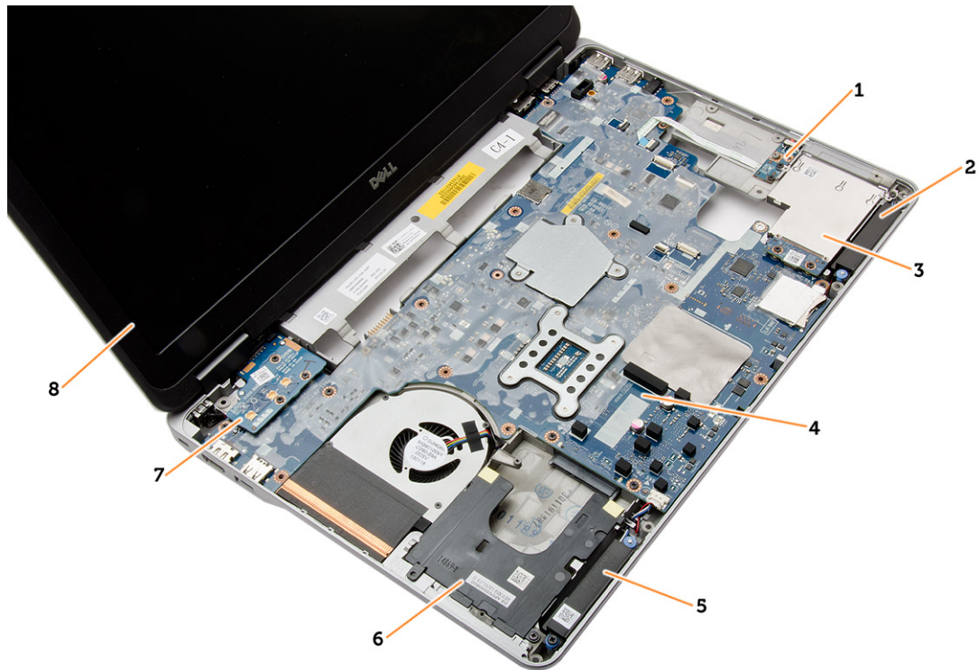
Figure 2. Top View — Keyboard and Palmrest Assembly removed
