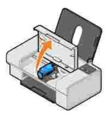
The ink cartridge carrier moves and stops at the loading position unless the printer is busy.
