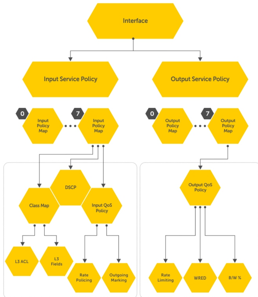
Figure 114. Constructing Policy-Based QoS Configurations
