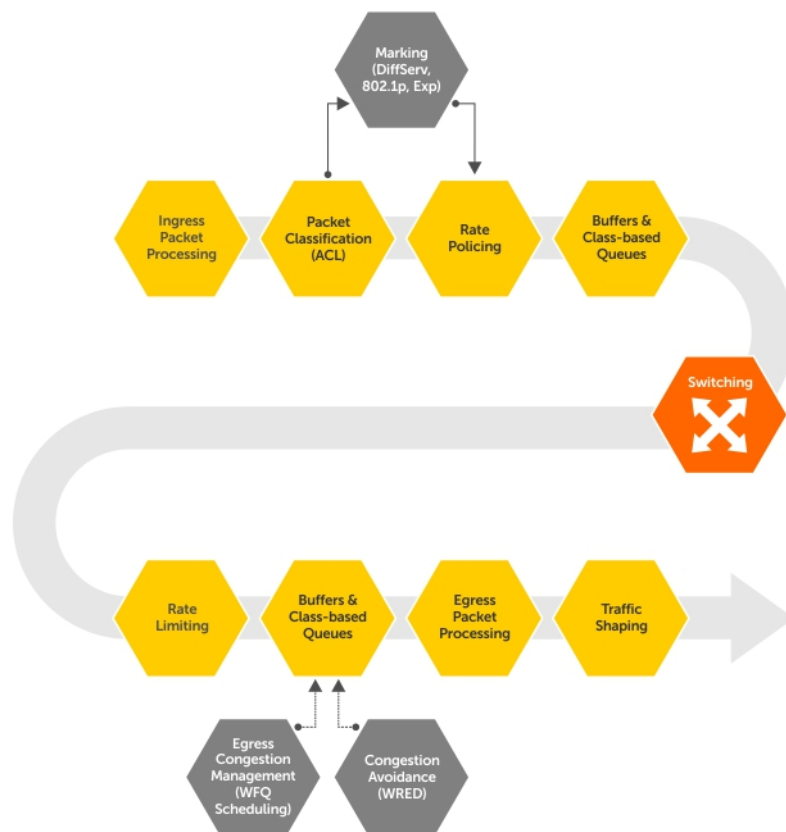
Figure 113. Dell EMC Networking QoS Architecture
