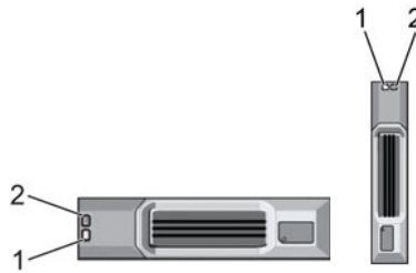
Figure 8. SCv300 and SCv320 Expansion Enclosure Drive Indicators
