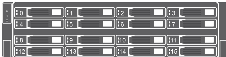
Figure 9. SCv3000 Storage System Drive Numbering
