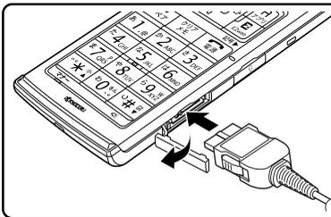
You can also connect the common AC adaptor 01/02 (option) to the W62K directly to charge the battery pack.
