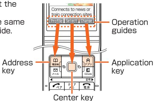
Various functions are assigned to the 3 keys depending on the screen in operation.
