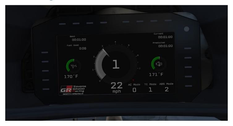
The Toyota GR86 uses a single-page, dash mounted display to show all engine data and race information to the driver in a clear and easy-to-read format.
