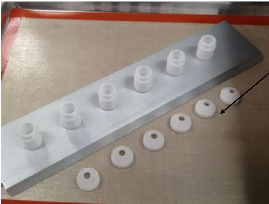
G. Remove nozzle tips by unscrewing.
