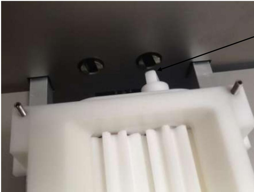
H. Remove pump by sliding out from the machine
