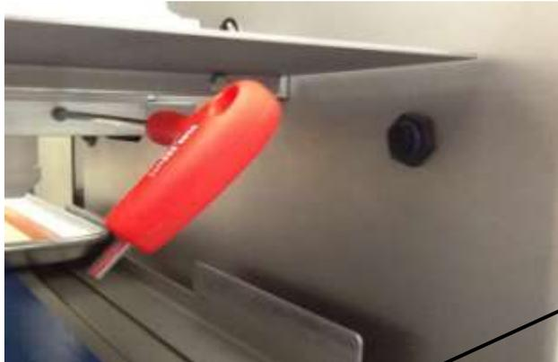
D. Remove white plastic spacer bar, by sliding it out.
