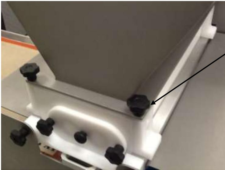
A. Remove hopper by unscrewing the black star knobs
