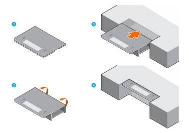
Figure 12. Installing the Service Baffle
