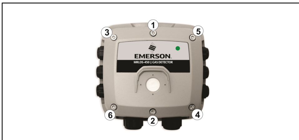
Figure 5 - Tightening Pattern
