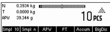
Press the «**Accum**» softkey to start the accumulation function.
