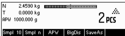
In this example, a reference weight determination has already been performed (Chapters 4.1.1 and 4.1.2).
