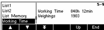
Press "Working Time". The working time, as well as the number of weighings will immediately be displayed on the right side of the screen.
