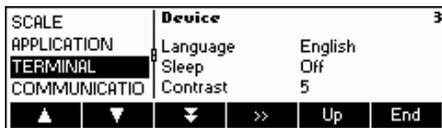
Select **TERMINAL** by pressing the «▼» key and press the «»» key.
