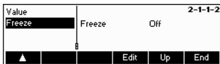
Choose "Freeze" and press «Edit». If this function is set to "On", it is no longer possible to change the value of Smpl X in Short Input Mode.
