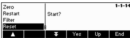
Press «**Yes**» to reset the scale settings. 'SURE?' will appear, press «**Yes**» to confirm. The scale settings are now reset to its original factory settings.
