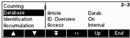
Press «>>>» to go to database settings menu. Select the item that you wish to modify by using the «▼» and «▲» softkeys. When the desired item is highlighted, press «>>>» to modify the item.
