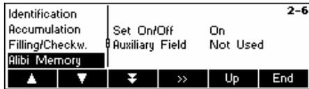
Select "on" or "off" for activating/deactivating the alibi memory. Apart from the mandatory fields one additional field for additional data can be defined. 150.000 weighings can be memorized in total.
