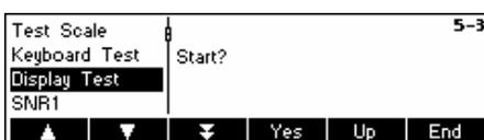
In order to check if the screen is functioning properly, press «**Yes**» and...
