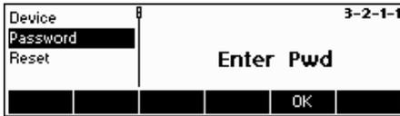
Enter the password using the keypad, press **«Ok»** to confirm. 'Retype Pwd' appears. Retype the new password and press **«Ok»** again.
