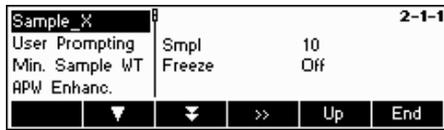
Press «>>>» to change the settings into the desired number of pieces or to freeze the actual setting of the Smpl X value.
