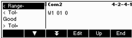
Choose **< Range-**, **< Tol-**, **Good**, **> Tol+**, **>Range+**, **Output off** or **Reset I/O** and then press the **«Edit»** softkey to define the commands.
