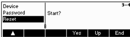
Press **«Yes»** to reset the terminal settings. 'SURE?' will appear, press **«Yes»** to confirm. The terminal settings are now reset to its original factory settings.
