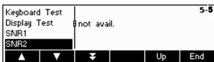
The **serial number** of the analog second scale, if installed, is displayed.
