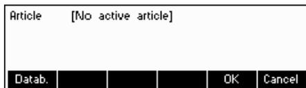
If in the "Vision Setup → APPLICATION → Database" the ID overview is set "On", you will enter a submenu into the database in which you can define additional information/identification. (Please view chapter 5.5.2 for the use of the IDs).
