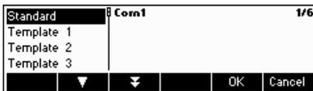
IND465 gives you the possibility to generate up to five different user-defined templates for your individual printouts. However, this must be set in "Vision Setup → COMMUNICATION → Define Printer" as described in Chapter 5.9.6.
