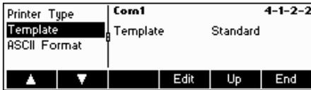
In case you want to use "Template" in your printouts, you may also assign this to the corresponding data interface. Choose "Template" and press **«Edit»**. (Templates can be created in "Vision Setup" menu under "COMMUNICATION → Def. Printout")
