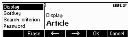
**Note:** Press the «Erase» softkey to clear the existing text and type the desired text using the keypad. Press the «→» and «←» keys to move cursor from left to right and vice-versa. Press «OK» when input is done. To deactivate the ID's, make their "Softkey" text blank (i.e. Press «Erase» then accept the empty text by pressing «OK»).
