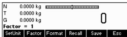
From the main Custom Unit screen you can define the text for the custom unit, set the factor to use for weighing, recall previous definitions, or save the current definition.
