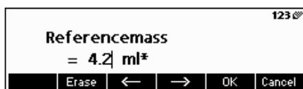
To use the automatically calculated factor, place the sample on the scale, press the «**Build**» softkey and enter the reference mass.
