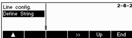
Choose "Define String" and press the «>>>» softkey to enter a text that you can define freely in "Text 1" and "Text 2", which can then be displayed on the fourth Info Line.
