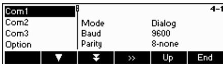
Select the COM port where you have connected your printer in "Vision Setup" menu under "COMMUNICATION". In our example, COM Port 1 (COM1) is used. Press «>>».
