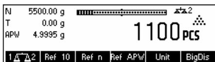
**Bulk** The second scale is to be used as bulk weight only. The APW will be calculated using the weight placed on the first scale (IND465 system), regardless of the active scale, then the weight on the second scale will be used for counting. This is used if the sample to be weighed is heavier than the maximum load of the IND465 system.
