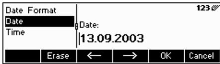
Use the numeric keypad to enter the date and confirm with the «OK» key. Incorrect inputs can be deleted with the «Erase» key. The «←» and «→» keys can be used to scroll the characters that are entered.
