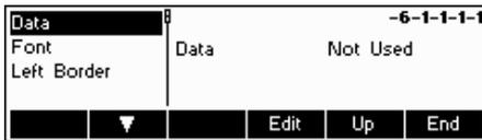
Choose "Date" to define the desired information for the line that was chosen. A detailed list of all functions can be found on the menu diagram (see Chapter 5.3.4 "COMMUNICATION → Def. Heading Line → Template 1-5 → Edit → Line 1-23 → Data").
