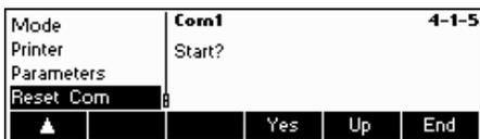
Press **«Yes»** to reset the settings of the current Com port. 'SURE?' will appear, press **«Yes»** to confirm. The chosen Com port is now reset to its original factory settings.
