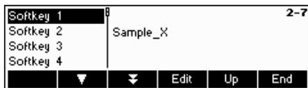
Select the desired softkey that is to be defined and press «Edit» to designate its function. It is possible to define up to 30 softkeys.
