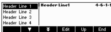
Choose the heading line to be edited and press «Edit». Using the keypad or a connected keyboard, enter the texts for the heading line.
