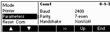
Go back one step back to the menu by pressing **«Back»** and then choose "Parameter". You may now change the settings for baud rate ("Baud"), parity and handshake. See the user's manual of your printer and verify the correct data. In our example, the value of the left picture to be made visible is turned on.
