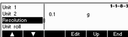
In order to change the settings of the resolution of the scale, select "Resolution" (this function is not available on all models).
