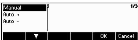
**Manual** - Perform the accumulation manually by confirming with the «+» or «-» key.
