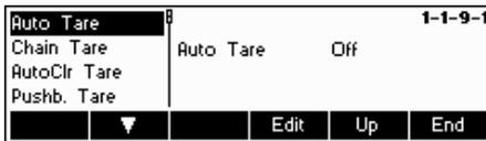
Switch the available functions **Auto Tare**, **Chain Tare**, **AutoClr Tare** or **Pushb. Tare** either On or Off.
