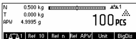
**Reference** The second scale is to be used for reference weight determination only. The APW will be calculated using the weight placed on the second scale regardless of the active scale. This is used if the second scale has a finer resolution than the IND465 system to achieve a more precise piece weight.
