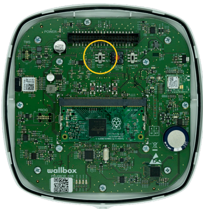
Fig. A3.1 Setting the RS485 switch to “T”
