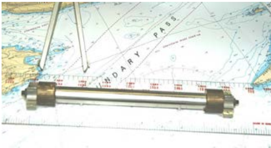
Figure 18 Measuring the Distance Between Gowlland Pt. and Sandy Pt. Step 5
