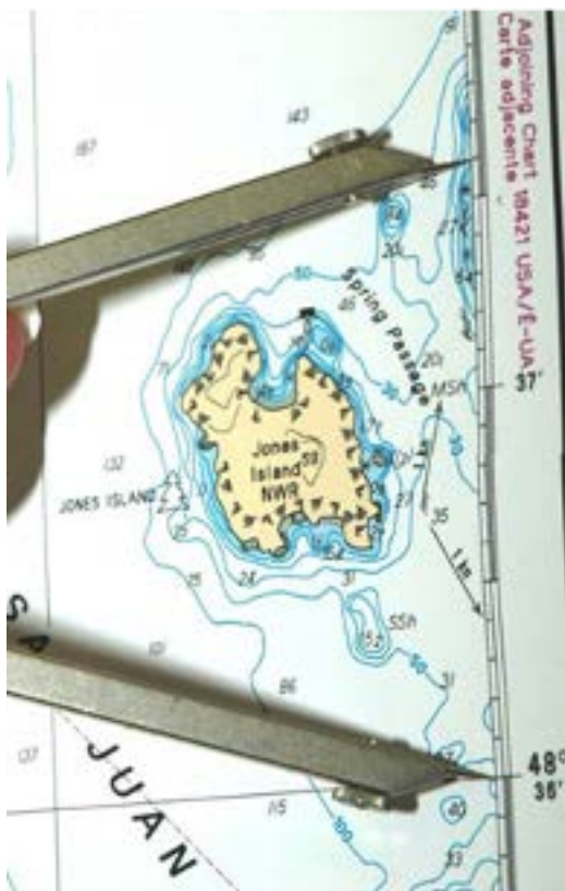
Figure 24 Plotting a Position (Method Two) Step 2
