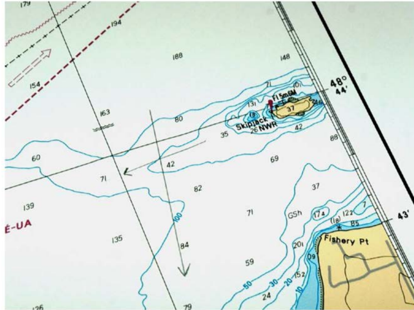
Figure A-1 Three-Bearing Fix Step 4
