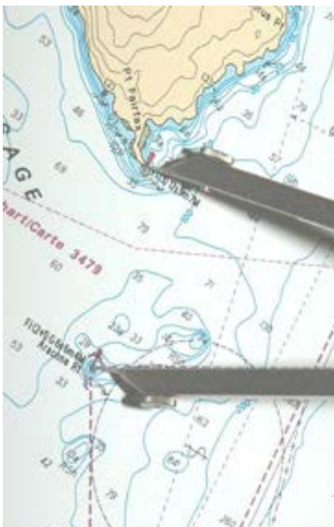
Figure 14 Measuring the Distance Between Arachne Rf. and Pt. Fairfax Step 2
