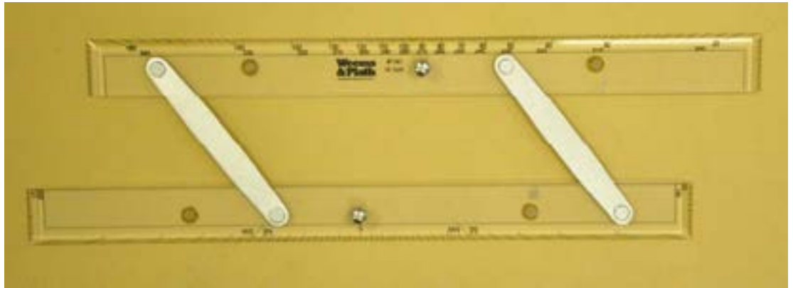
Figure 1 Hinged Parallel Ruler
