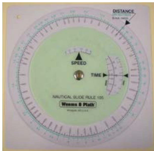
Figure 5 Weems & Plath Speed-Time-Distance Calculator
