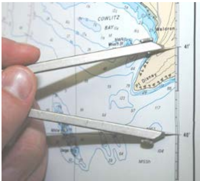
Figure 16 Measuring the Distance Between Gowlland Pt. and Sandy Pt. Step 1
