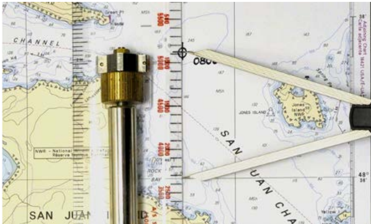
Figure 25 Plotting a Position (Method Two) Step 6
