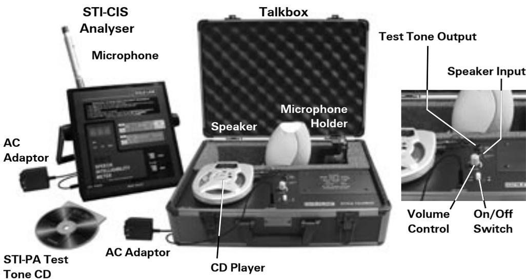
Figure 2. Equipment required to Measure Speech Intelligibility
