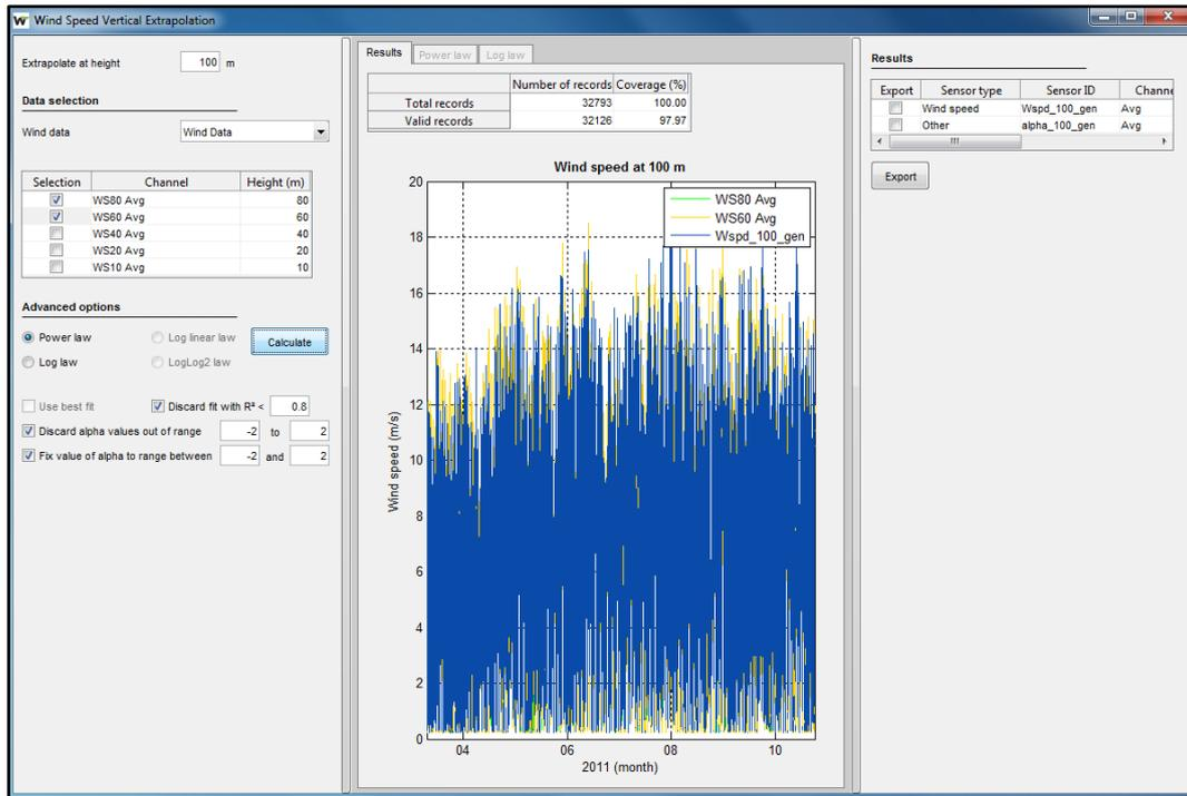
Figure 46: Wind speed vertical extrapolation module with 2 channels
