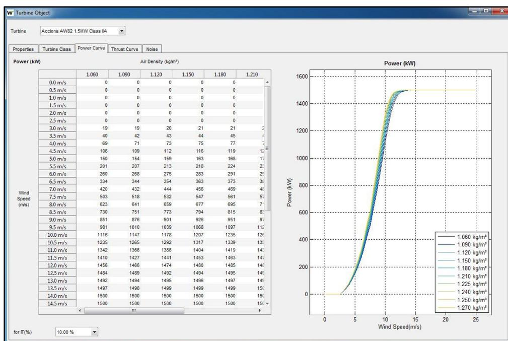
Figure 120: Example of wind turbine power curve
