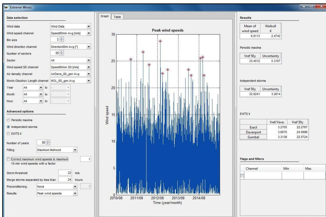
Figure 62: Extreme winds module using Independent storms method
