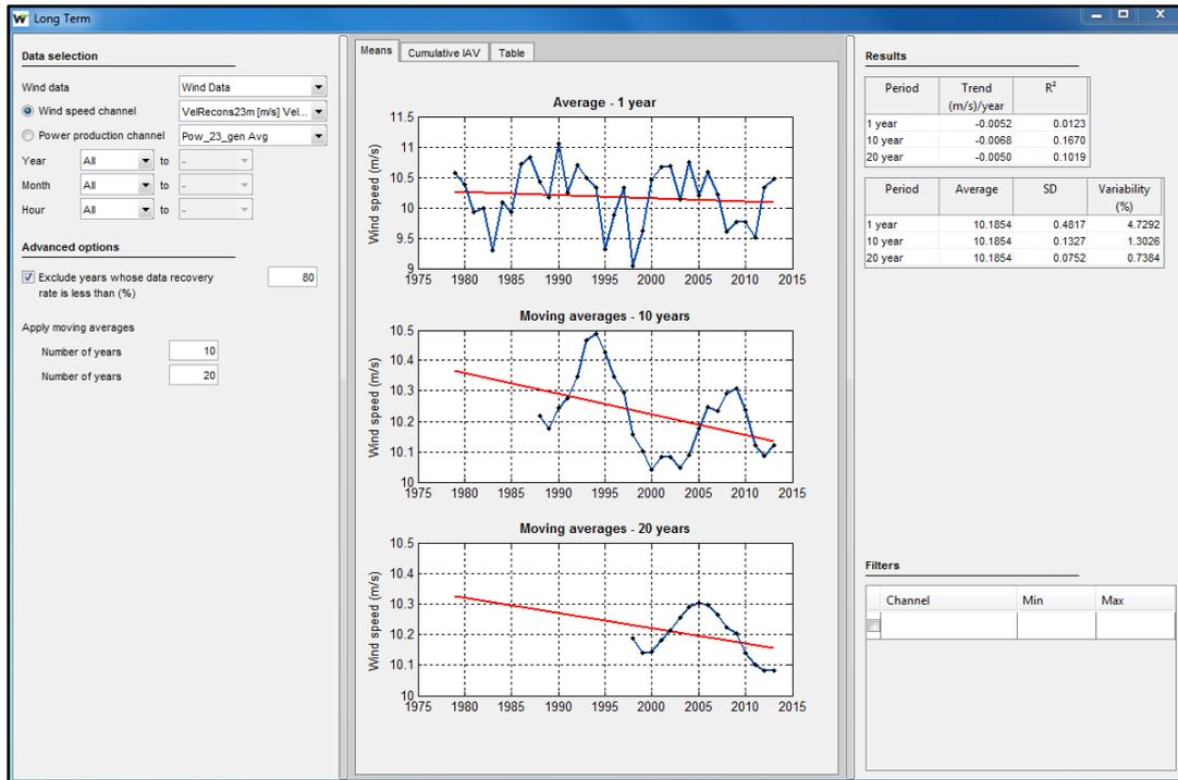
Figure 60: Long term module for wind speed channel
