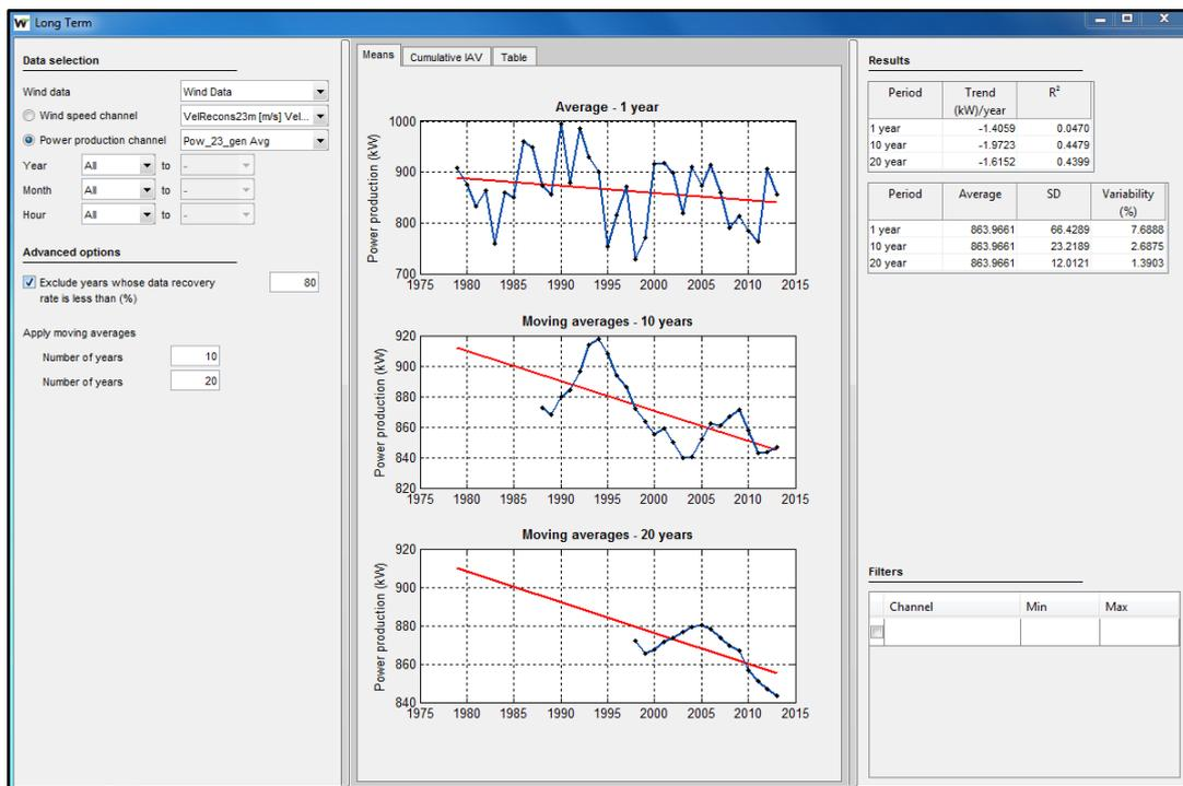
Figure 61: Long term module for power production channel
