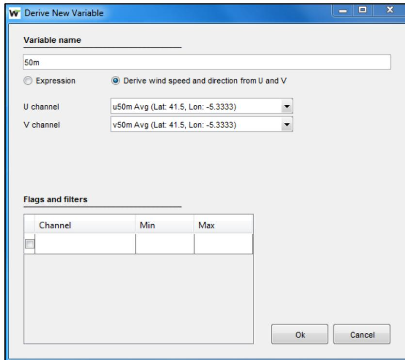
Figure 44: Derive new variable module for U and V
