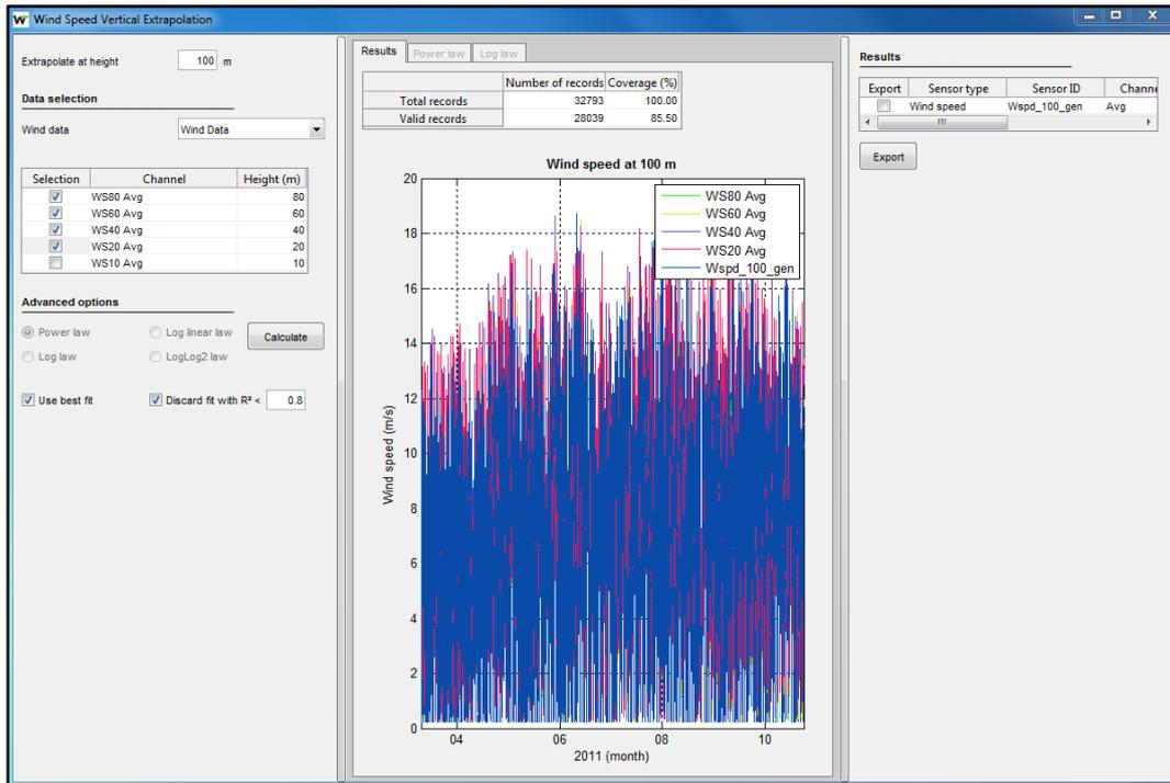
Figure 47: Wind speed vertical extrapolation module with 4 channels
