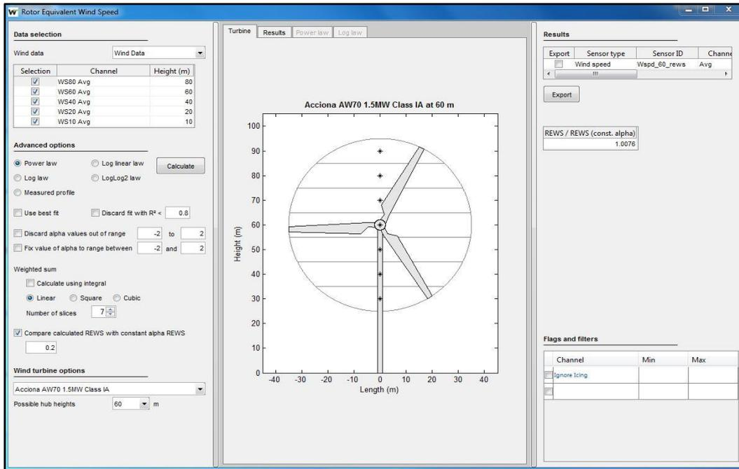
Figure 50: Rotor equivalent wind speed module
