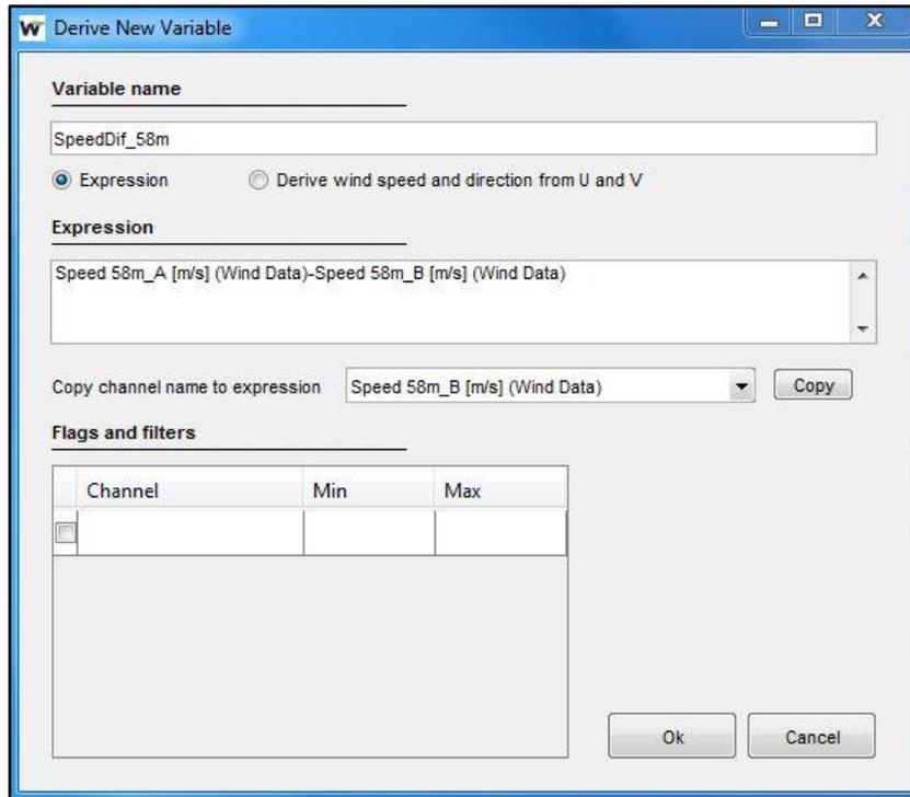
Figure 43: Derive new variable module
