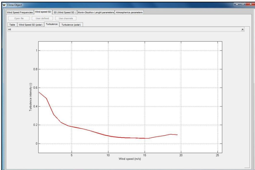
Figure 80: Turbulence intensity distribution for the CLIMA object
