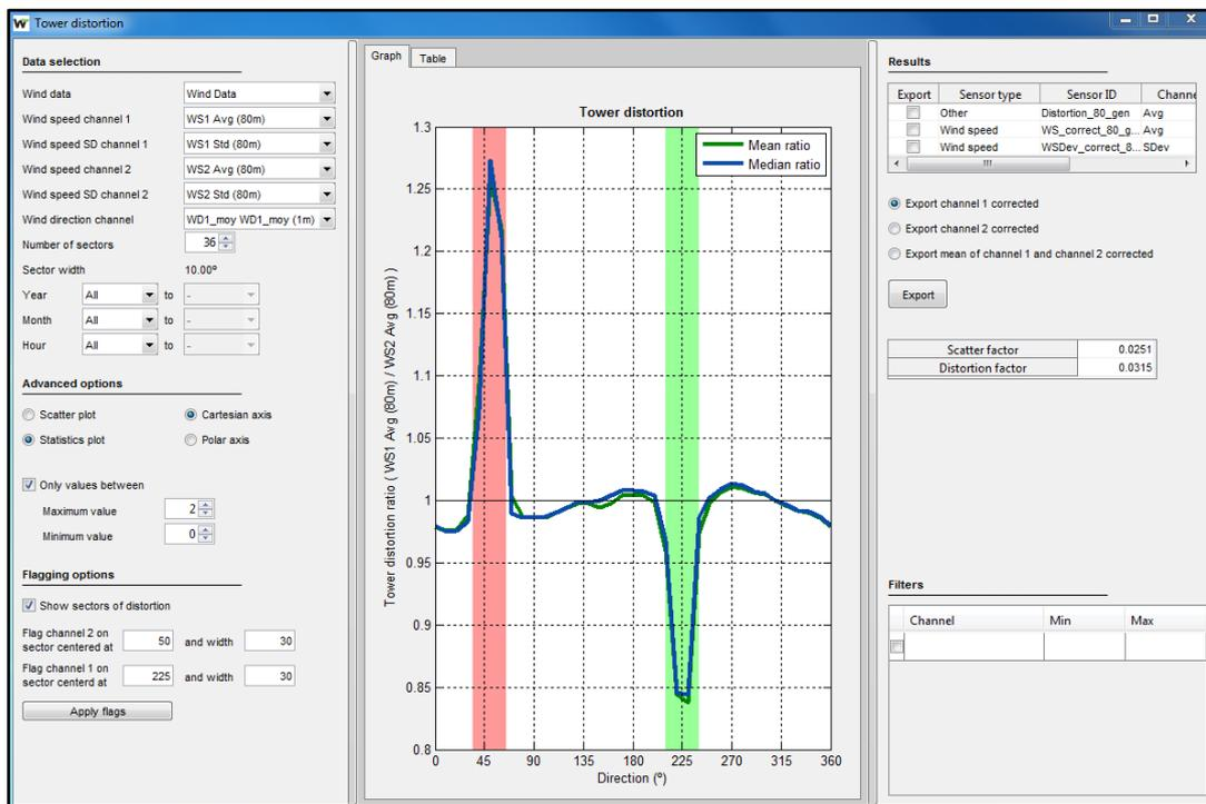
Figure 42: Tower distortion module
