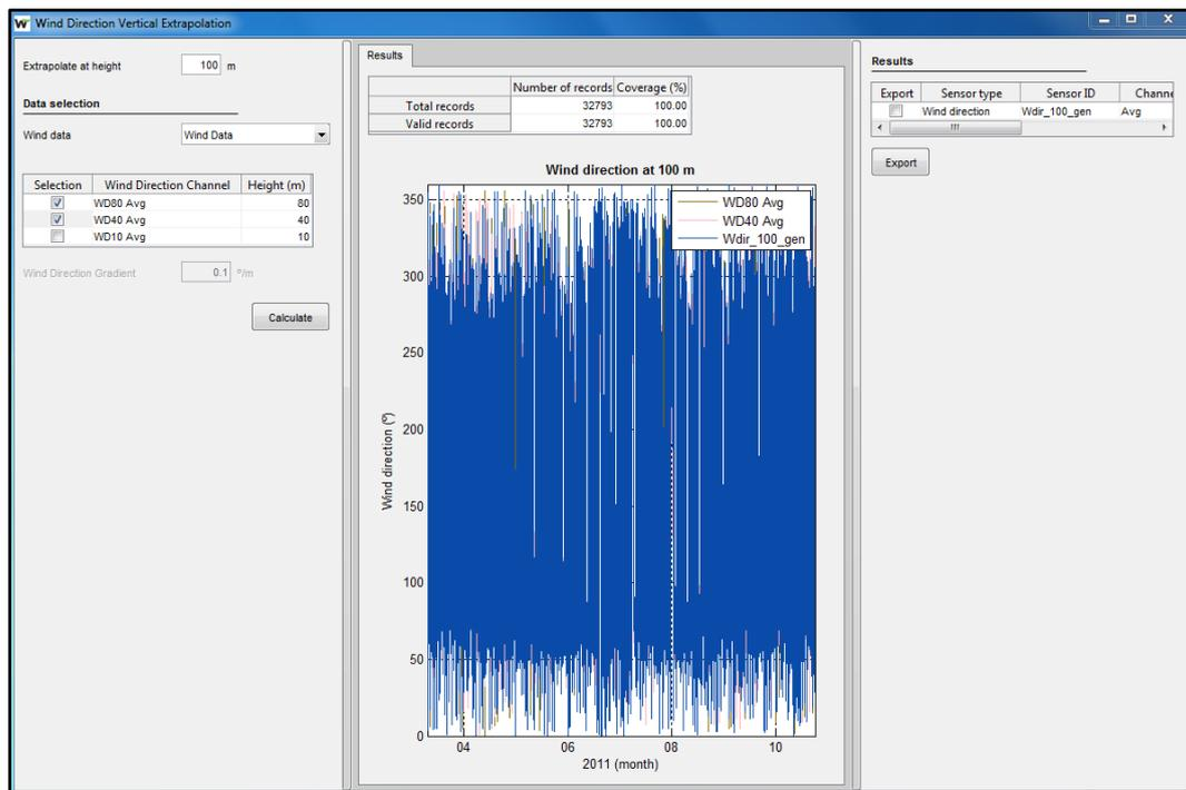
Figure 48: Wind direction vertical extrapolation module
