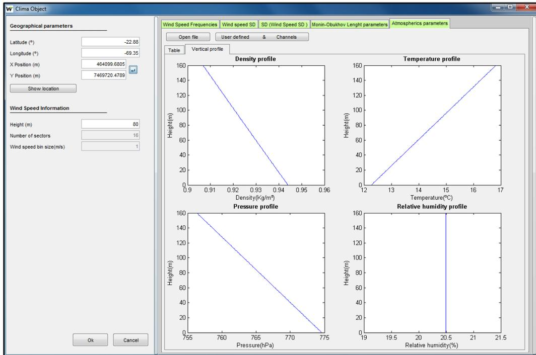
Figure 78: Vertical profile of each atmospheric variable
