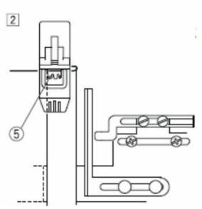
3. Slide the cover hem guide and align the guide step with the raw edge then tightenthe two setscrews securely.(6) Guide step
