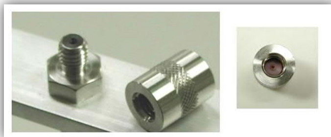
Figure 116: Septum Nut with used septum
