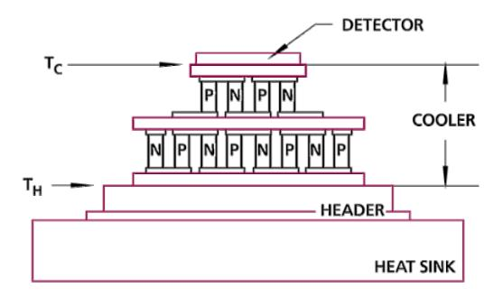
In TE cooled detectors, cooler performance can be characterized by the required input power to achieve the  $\Delta T$  required where  $\Delta T = T_H - T_C$ ,  $T_H$  is the ambient or heat sink temperature and  $T_C$  is the cold plate temperature (See Fig. below).
