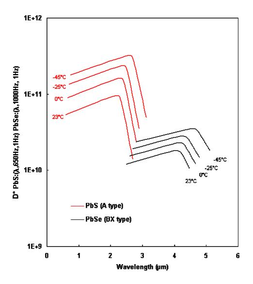
By altering controlled chemical deposition parameters, Cal Sensors can consistently produce detectors with very high peak detectivity or extended wavelength response at a given operating temperature. Cooling shifts both the spectral response and cutoff wavelength of PbS and PbSe detectors to longer wavelengths.
