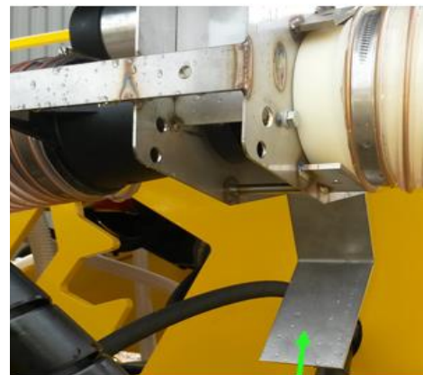
Figure 30.2 - Hinged flap open for metering out product
