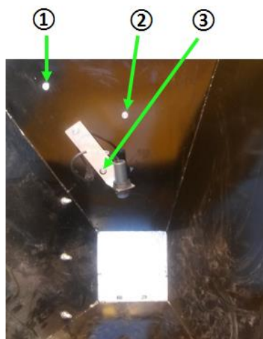
Figure 27 - Level sensor in lower position
