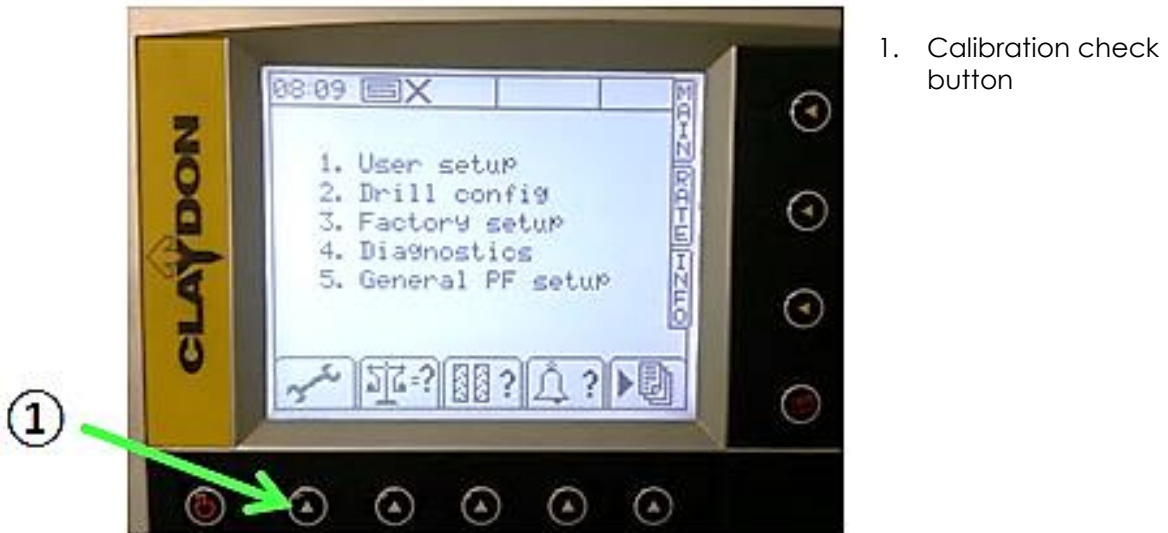
Figure 36 – Calibration check option
