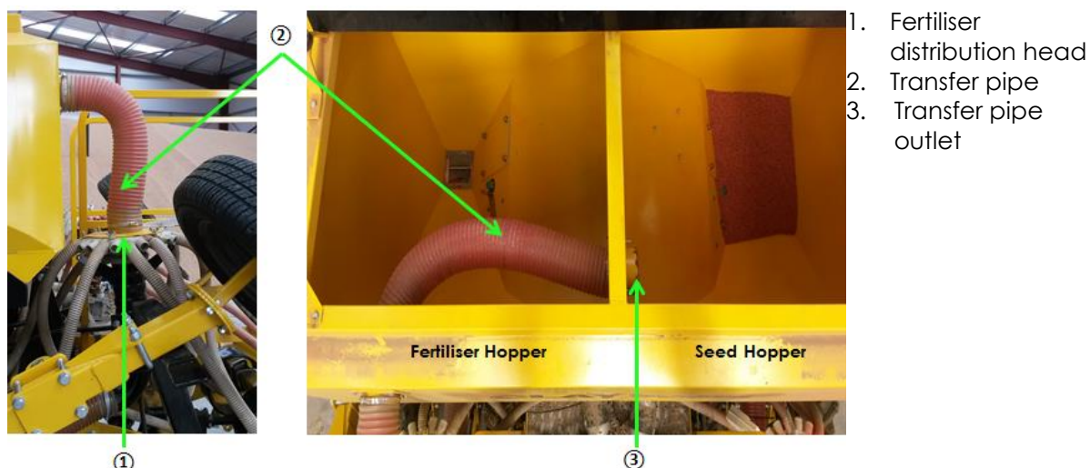
Figure 52 – Hopper to Hopper Transfer kit Installed
