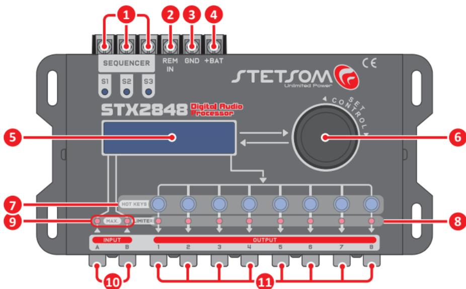
**1. SEQUENCER:** It allows sequential activation of other products through the remote activation (REM) connection. Use a cable of at least **AWG 20**.
