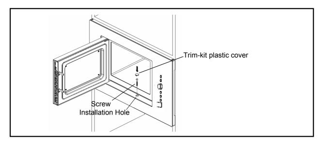
2. Open the door; fix the oven to the cabinet with SCREW at the INSTALLATION HOLE of TRIM KIT. Then fix the TRIM-KIT PLASTIC COVER to the INSTALLATION HOLE.
