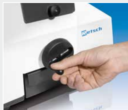
Setting the gap width to determine the final fineness
