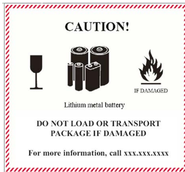
Figure 1 Lithium Battery Handling Label
