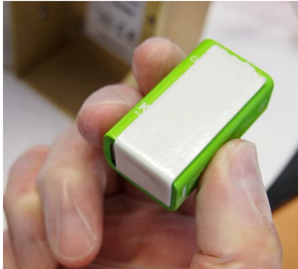
Figure 32 Two-Sided Tape Attached to the Battery
