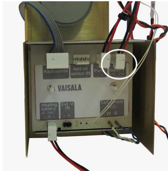
Figure 28 Connecting Ozone Sensor Battery Cable
