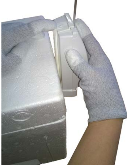
Figure 43 Pushing the Holder into Place
