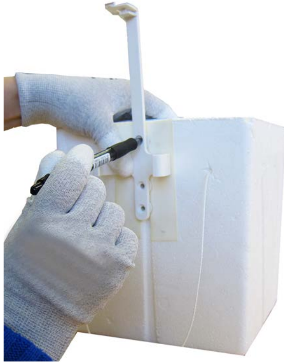
Figure 16 Marking the Positions of the Holder Screws
