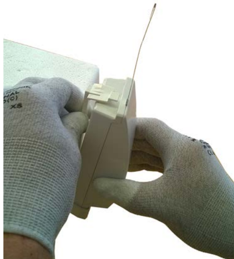
Figure 42 Attaching Radiosonde to the Holder
