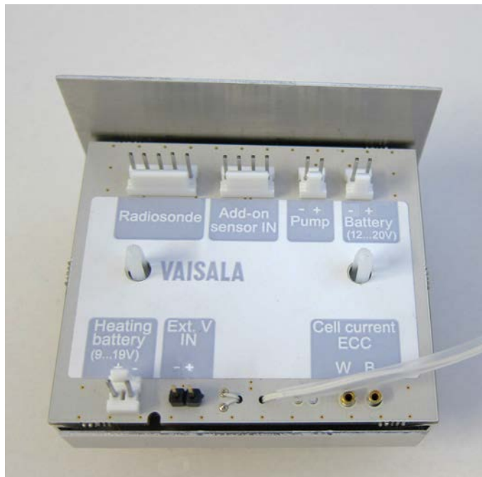
Figure 4 Ozone Sensor Interface Board OIF411
