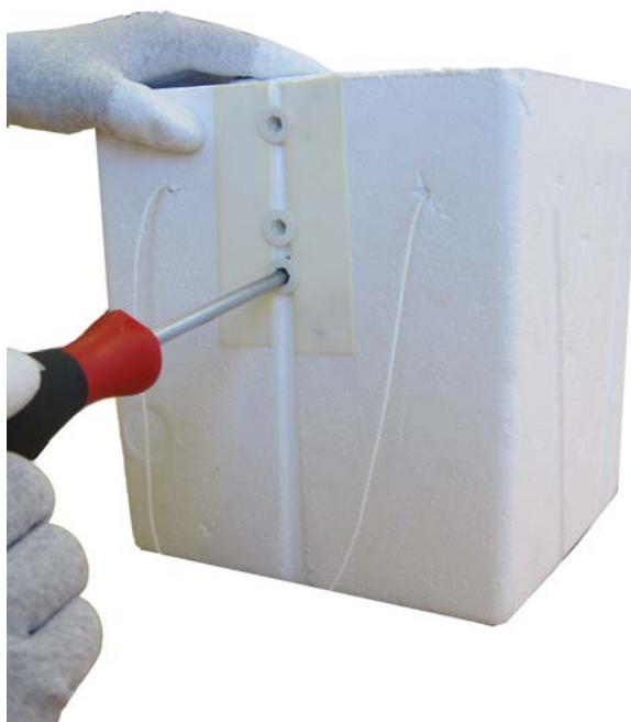
Figure 17 Inserting the Dowels
