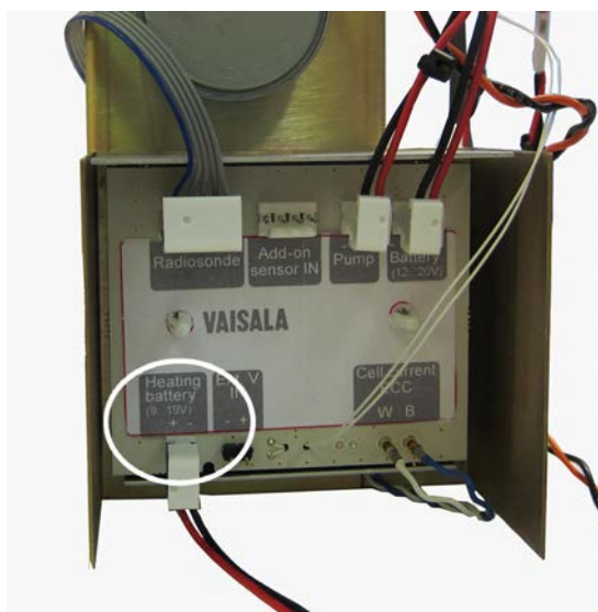
Figure 31 Connecting Heating Battery
