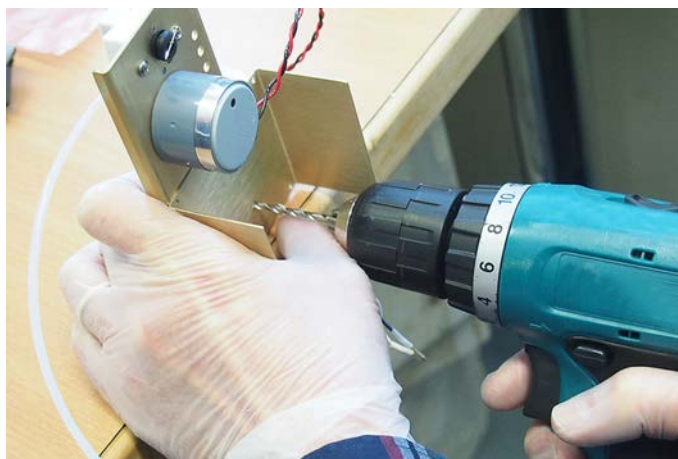
Figure 23 Drilling the Ozone Sensor Frame Holes
