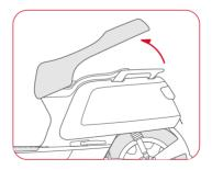
Open the saddle to take out the key box, windshield package (with rubber pads and standard parts), and installation tools
