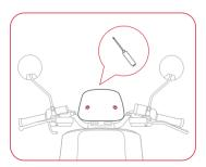
Step 5 Align the windshield rubber part with the windshield holes and then install it.
