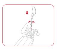
Take out the rearview mirrors and check them carefully. Install the left rearview mirror into the mounting hole on the left brake lever and turn it clockwise. The bolt shall be screwed in for more than 15 mm
