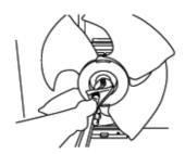
2) Loose 2 screw fixing the fan motor angle.
