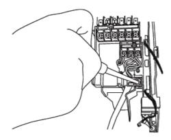
4) Remove a screw fixing the Cord holder and 2 screw fixing the Terminal board.
