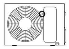
8) Loose 7 screws fixing the rear cabinet.
