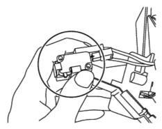
3) Remove a screw fixing the Cord holder.
