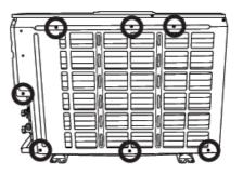
9) Loose 1 screw fixing the rear cabinet (left side).
