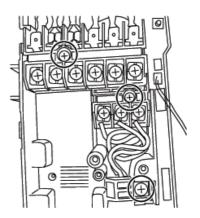
5) Remove 2 screws fixing the Transformer and pull the Control board unit.
