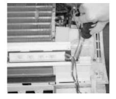
15) Remove the Drain cover from the Evaporator
