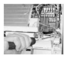
13) Remove 2 screws fixing the Control box and remove it.
