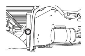
14) Loose 3 screws fixing the bulkhead.
