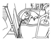
11) Loose 1 screw fixing the control box.
