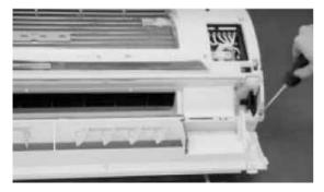
4) Remove the screw fixing the Cord holder.
