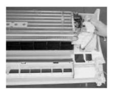
16) Remove 3 screws fixing the Evaporator.
