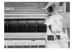
19) Loose a screw fixing Cross flow fan.
