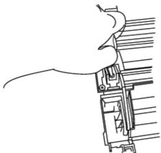
Remove the connector of louver motor and take off the wire and holder.
