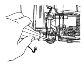
2) Remove the 2 Switch and Photo detector unit.
