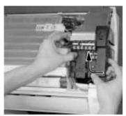
8) Cut the fixing band and remove the Cover B.
