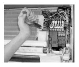
9) Remove a screw fixing the ground wire.
