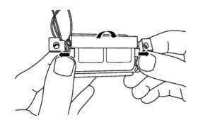
3) Remove the connector of high voltage unit ass'y.
