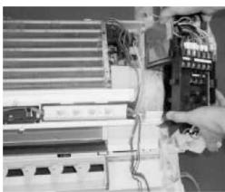
14) Remove a screw fixing the drain pan and pull Drain pan toward you.
