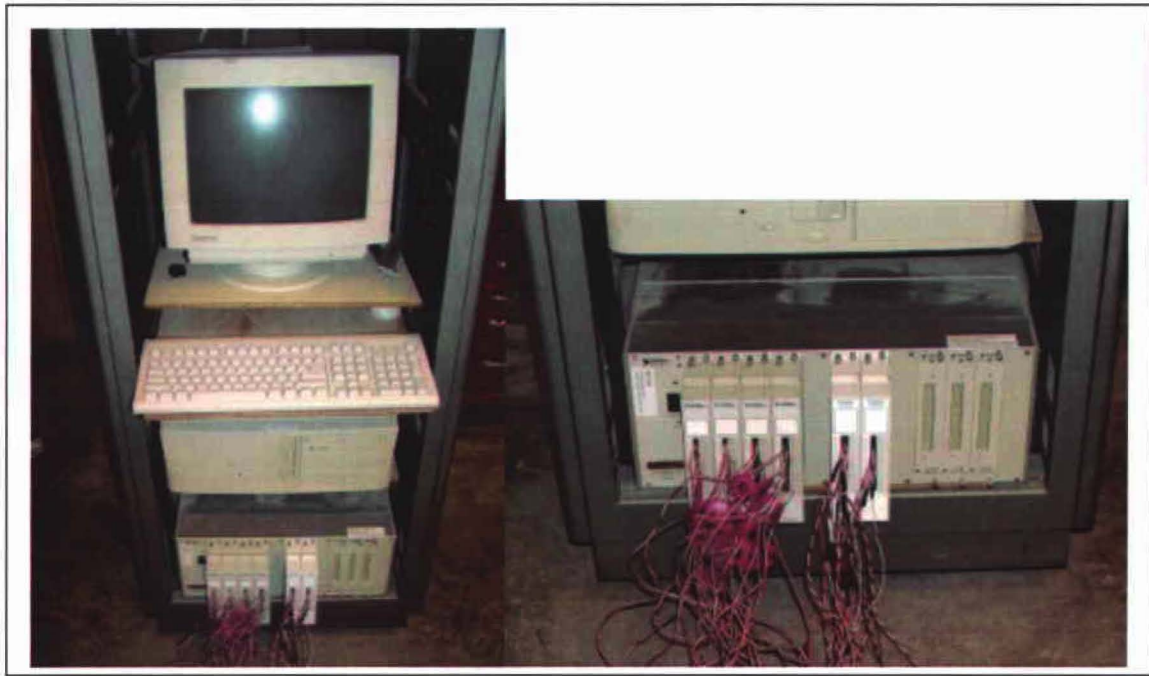
Figure 3-5: LabVIEW data acquisition system
