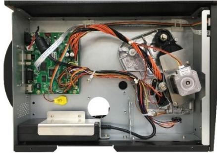
2. Remove the two screws on slot-in Wi-Fi/ GPIO interface board (if module installed).
